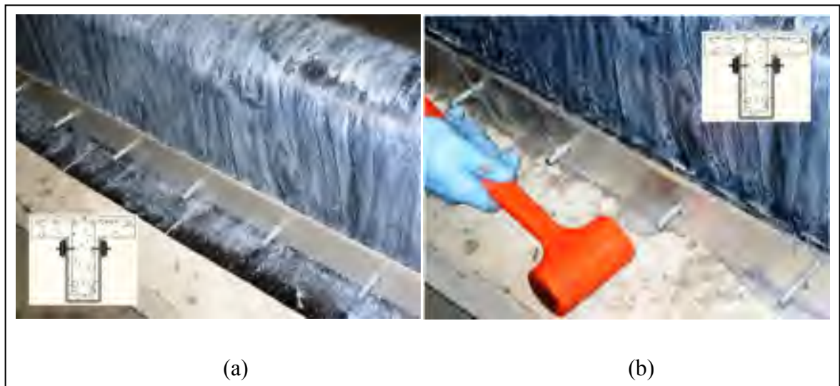
Figure 6.3 Elevation of specimen S3-EB-DAMA; a) first aluminum plate installed; and b) second aluminum plate installed
