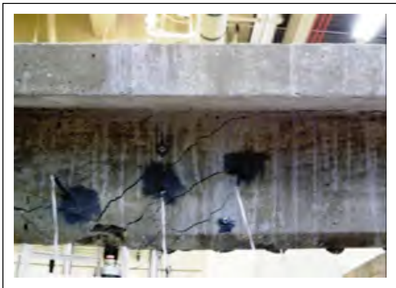
Figure 7.8 Failure mode of specimen S1-12d130s.
