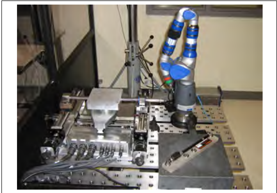
Figure 2.8 Experimental setup for calibrating the PreXYT with a FaroArm
