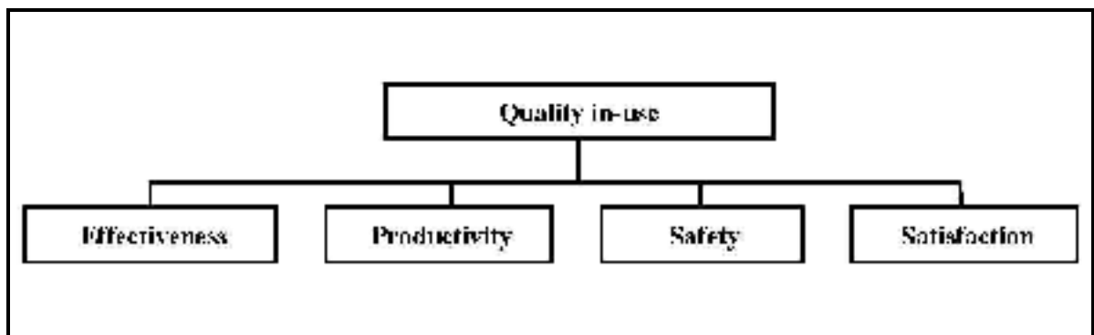
Figure 1.4 ISO/IEC 9126 Quality Model - Quality in Use Extracted from Suryn et al., (2005b)
