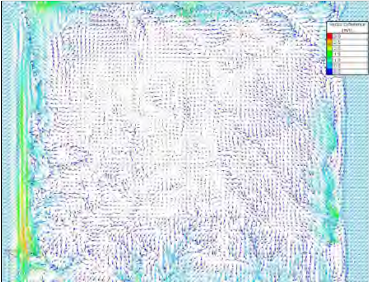
Figure 3.7 Vector difference of the simulated wind flow for the cases of “classification variant 2” with initial reference topography at 0m ASL and initial reference topography” at 600m ASL
