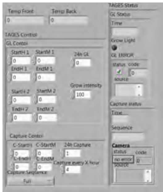
Figure 1.4 LabView TIS-III control panel
