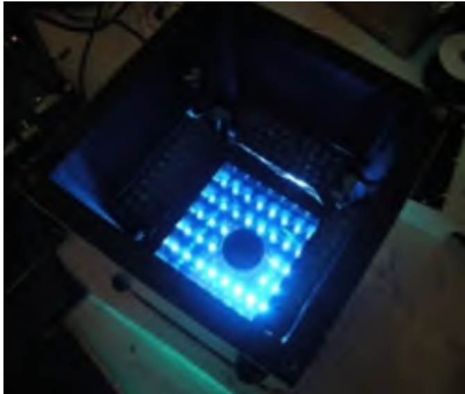
Figure 1.8 TIS-III excitation LEDs behind a band-pass filter
