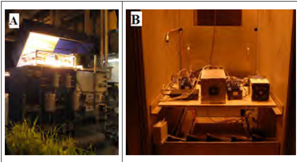
Figure 2.1 Canopy-scale hypobaric chambers at the Controlled Environment Systems Research Facility (CESRF), University of Guelph: A) Exterior showing lighting canopy, irrigation and nutrient control system, B) M-PHIS deployed in a CESRF hypobaric plant growth chamber
