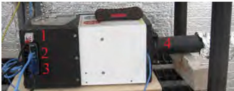
Figure 1.2 Side view of the TIS-III as installed. Grow lights and fan inputs (1), camera Ethernet connection (2), camera power cable (3), cooling pipe (4)
