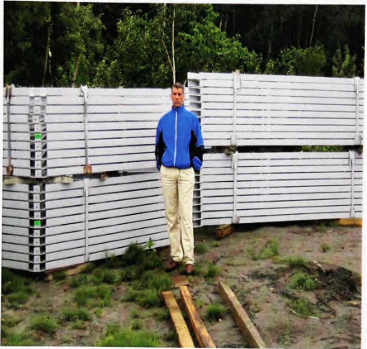
Frame components post fabrication at Air-Therm works scanned and approved for transport to jobsite
