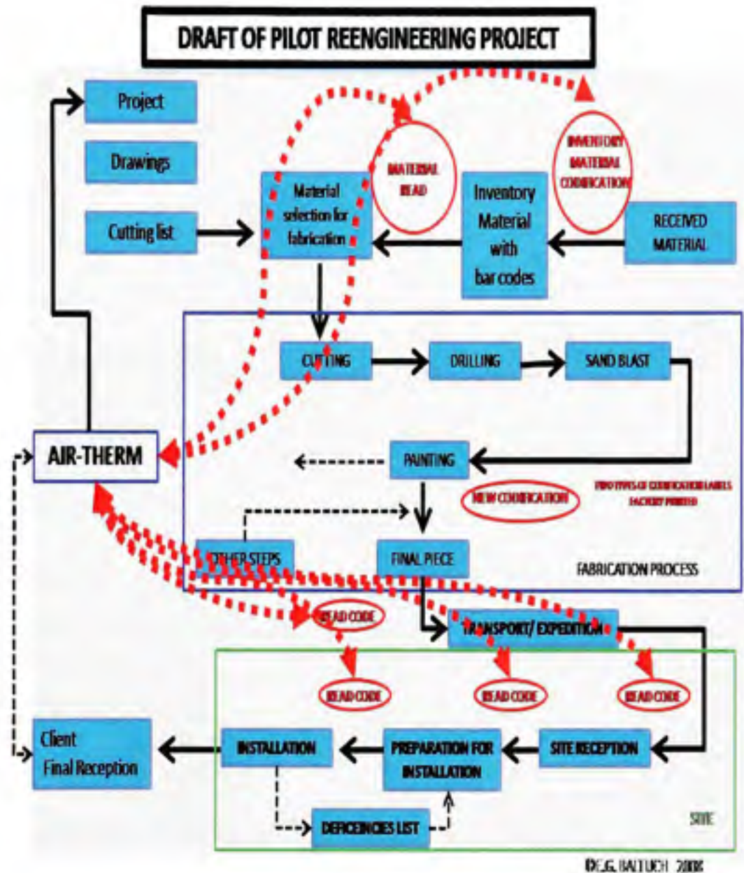
Figure 4.12 Pilot Re-engineering Project 4
