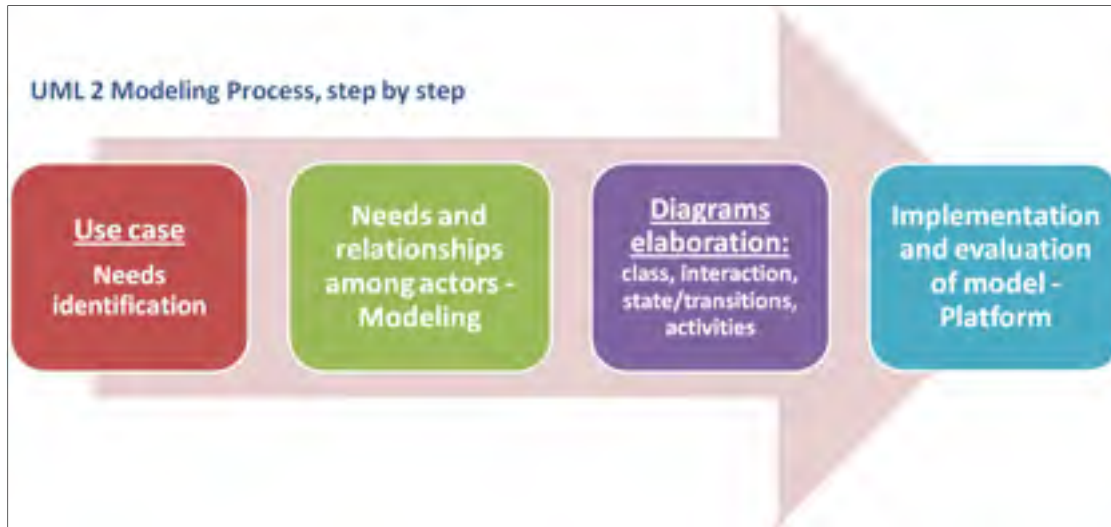
Figure 3.3 Step-by-step process to represent the collaborative platform Adapted from Charroux, Osmani and Thierry-Mieg (2008)
