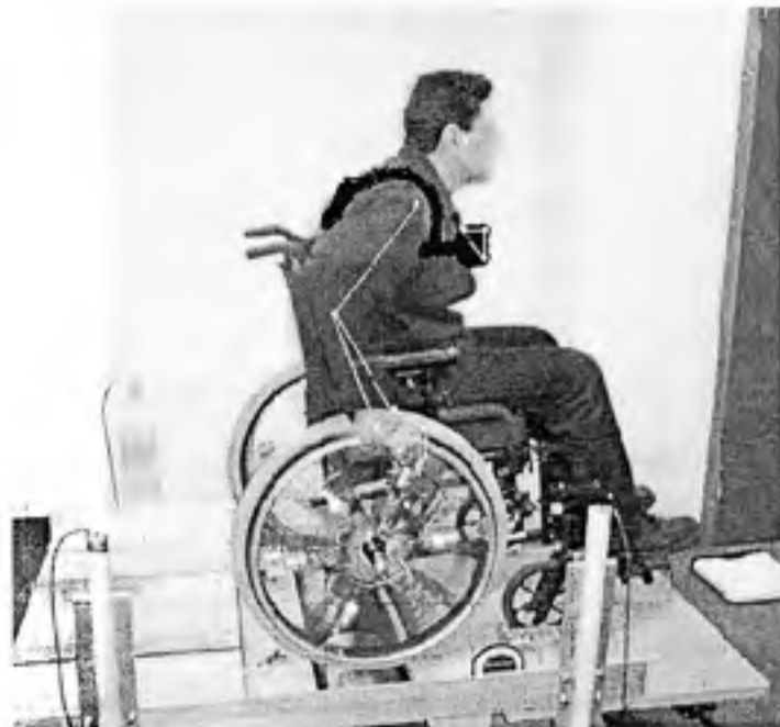
Figure 7.1 Subject propelling on the custom-built wheelchair that was fixed to the experimental ergometer.
