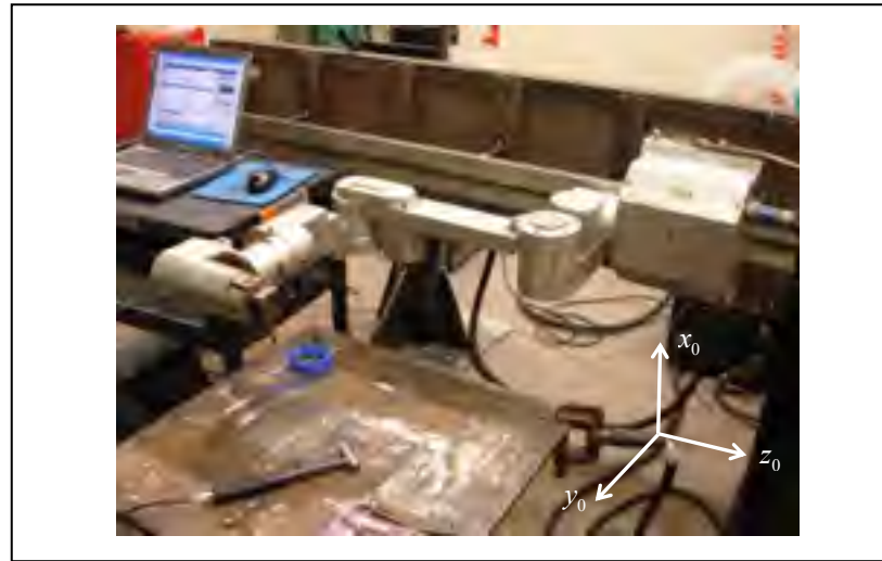
Figure 5.3 Configuration of SCOMPI for modal testing experiment
