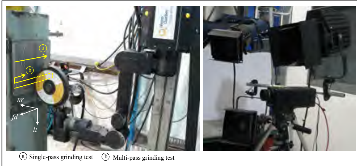
Figure 3.10 Robotic grinding test rig with high-speed camera and lighting
