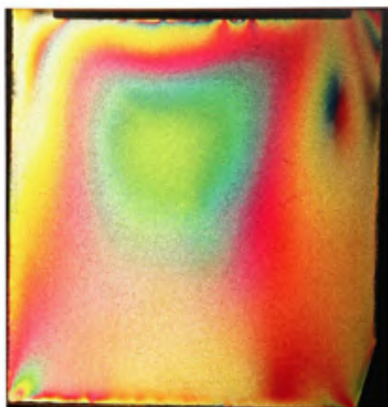
Figure II.26 Ft=17.8 , Fn=222.4 , Mat=PSI , Ang=75^\circ
