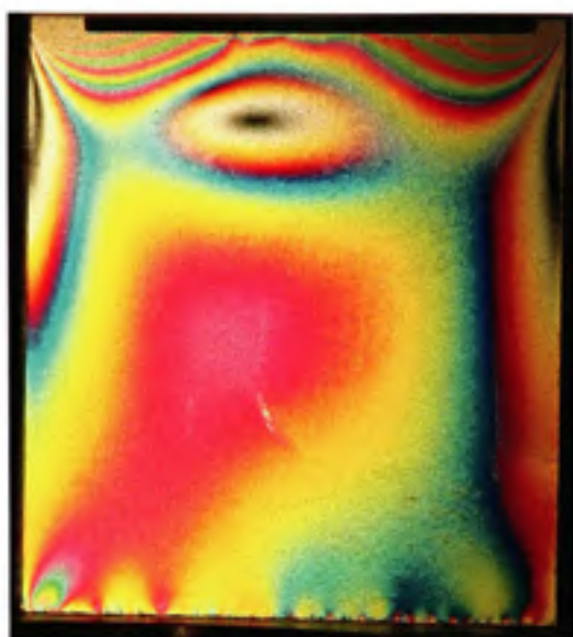
Figure II.7 Ft=8.9 , Fn=222.4 , Mat=Acier , Ang=90^\circ
