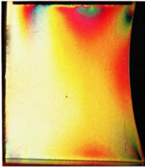
Figure II.67 Ft=8.9 , Fn=133.5 , Mat=Caout , Ang=105^\circ
