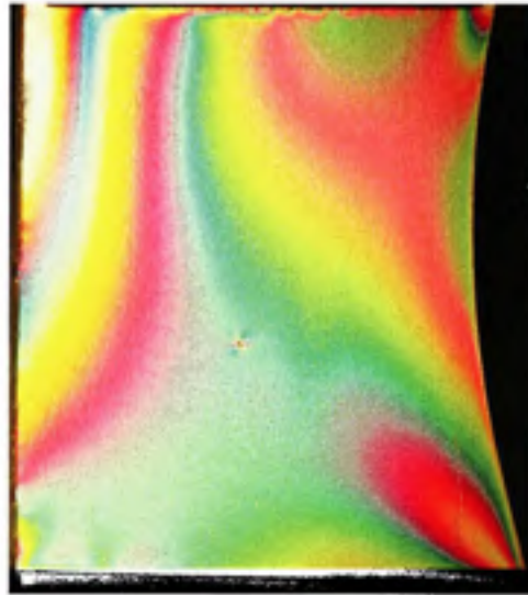
Figure II.75 Ft=26.7 , Fn=311.4 , Mat=Caout , Ang=105^\circ
