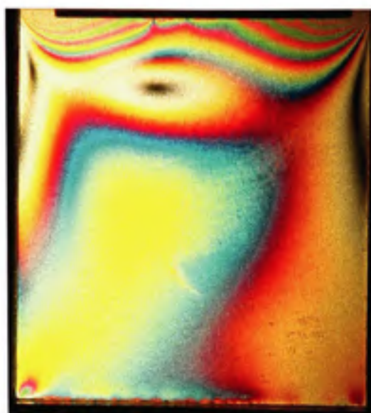
Figure II.31 Ft=8.9 , Fn=133.5 , Mat=PSI , Ang=90^\circ
