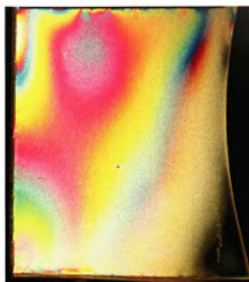
Figure II.14 Ft=17.8 , Fn=133.5 , Mat=Acier , Ang=105^\circ
