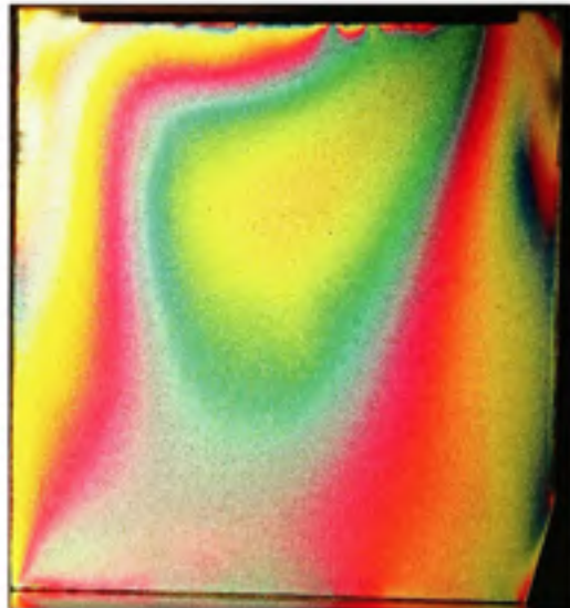
Figure II.57 Ft=26.7 , Fn=311.4 , Mat=Caout , Ang=75^\circ
