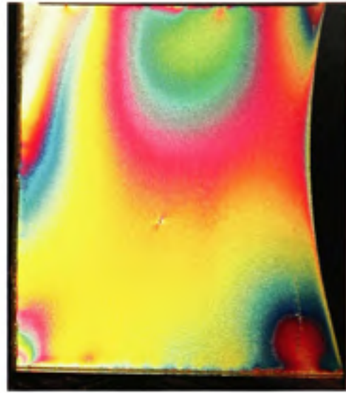
Figure II.44 Ft=17.8 , Fn=222.4 , Mat=PSI , Ang=105^\circ
