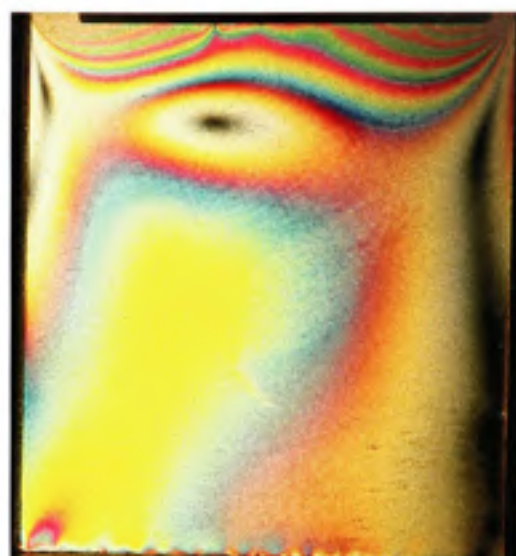
Figure II.5 Ft=17.8 , Fn=133.5 , Mat=Acier , Ang=90^\circ
