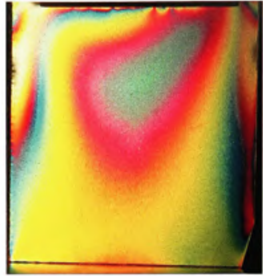
Figure II.53 Ft=17.8 , Fn=222.4 , Mat=Caout , Ang=75^\circ
