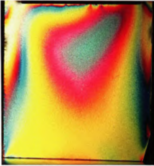
Figure II.52 Ft=8.9 , Fn=222.4 , Mat=Caout , Ang=75^\circ
