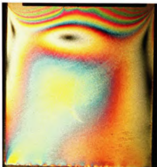
Figure II.4 Ft=8.9 , Fn=133.5 , Mat=Acier , Ang=90^\circ
