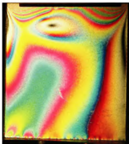
Figure II.9 Ft=26.7 , Fn=222.4 , Mat=Acier , Ang=90^\circ
