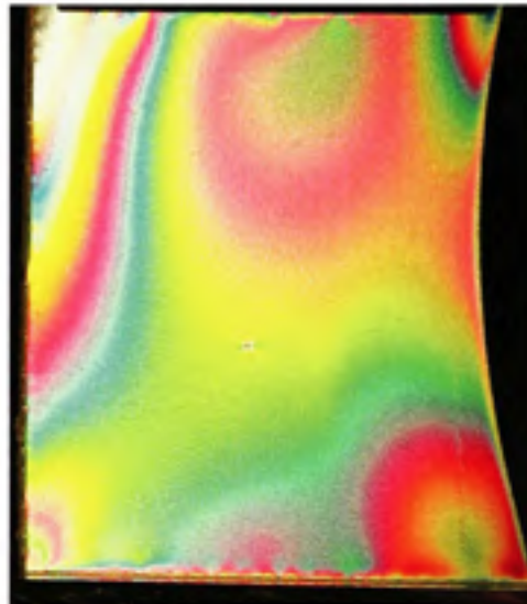
Figure II.48 Ft=26.7 , Fn=311.4 , Mat=PSI , Ang=105^\circ
