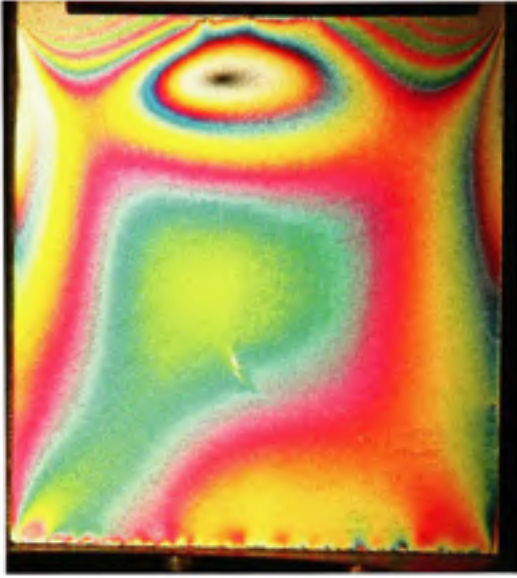
Figure II.10 Ft=8.9 , Fn=311.4 , Mat=Acier , Ang=90^\circ
