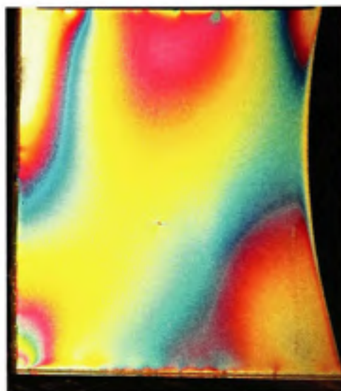
Figure II.42 Ft=26.7 , Fn=133.5 , Mat=PSI , Ang=105^\circ
