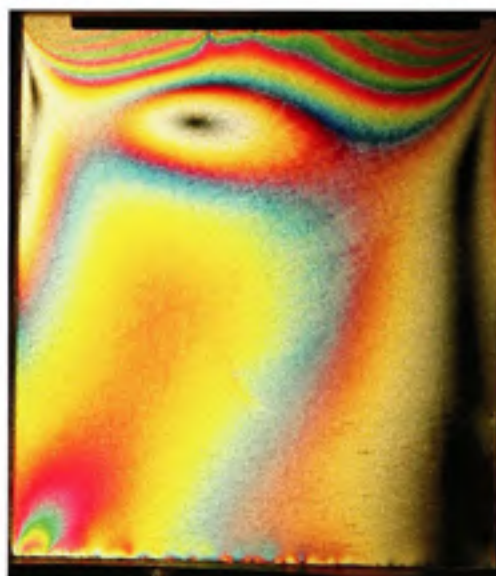
Figure II.4 Ft=8.9 , Fn=133.5 , Mat=Acier , Ang=90^\circ
