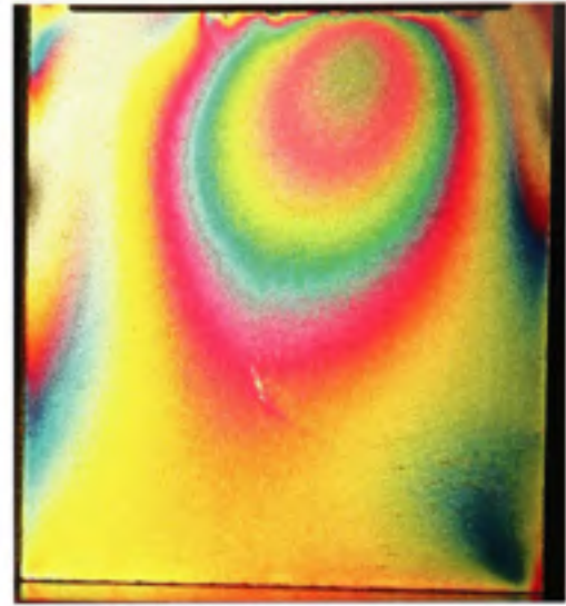
Figure II.62 Ft=17.8 , Fn=222.4 , Mat=Caout , Ang=90^\circ
