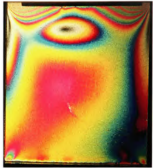
Figure II.35 Ft=17.8 , Fn=222.4 , Mat=PSI , Ang=90^\circ
