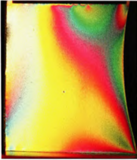
Figure II.70 Ft=8.9 , Fn=222.4 , Mat=Caout , Ang=105^\circ
