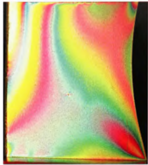
Figure II.74 Ft=17.8 , Fn=311.4 , Mat=Caout , Ang=105^\circ
