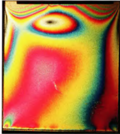
Figure II.36 Ft=26.7 , Fn=222.4 , Mat=PSI , Ang=90^\circ
