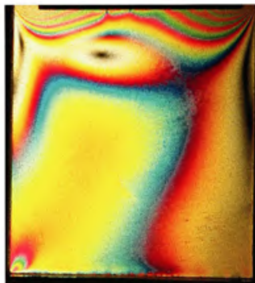
Figure II.33 Ft=26.7 , Fn=133.5 , Mat=PSI , Ang=90^\circ
