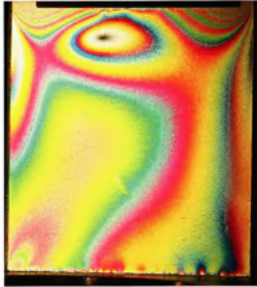
Figure II.12 Ft=26.7 , Fn=311.4 , Mat=Acier , Ang=90^\circ
