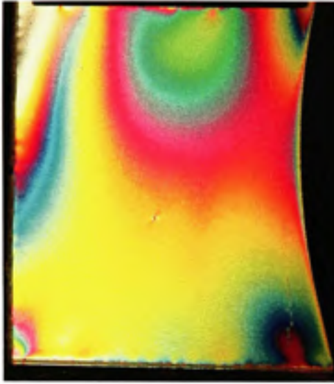
Figure II.43 Ft=8.9 , Fn=222.4 , Mat=PSI , Ang=105^\circ
