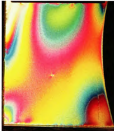
Figure II.45 Ft=26.7 , Fn=222.4 , Mat=PSI , Ang=105^\circ
