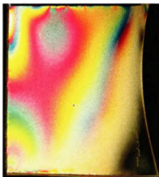
Figure II.15 Ft=26.7 , Fn=133.5 , Mat=Acier , Ang=105^\circ
