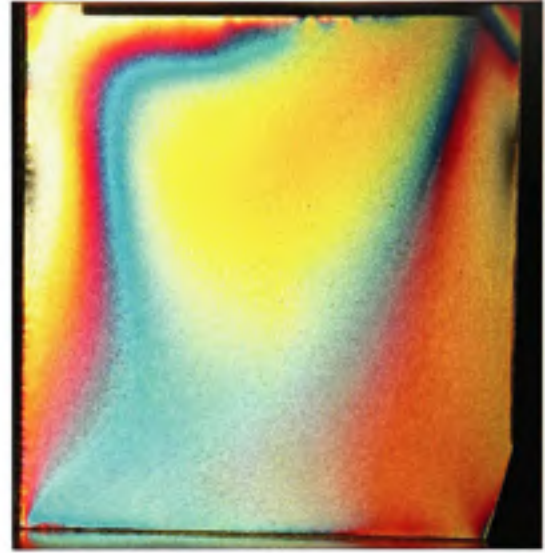
Figure II.50 Ft=17.8 , Fn=133.5 , Mat=Caout , Ang=75^\circ
