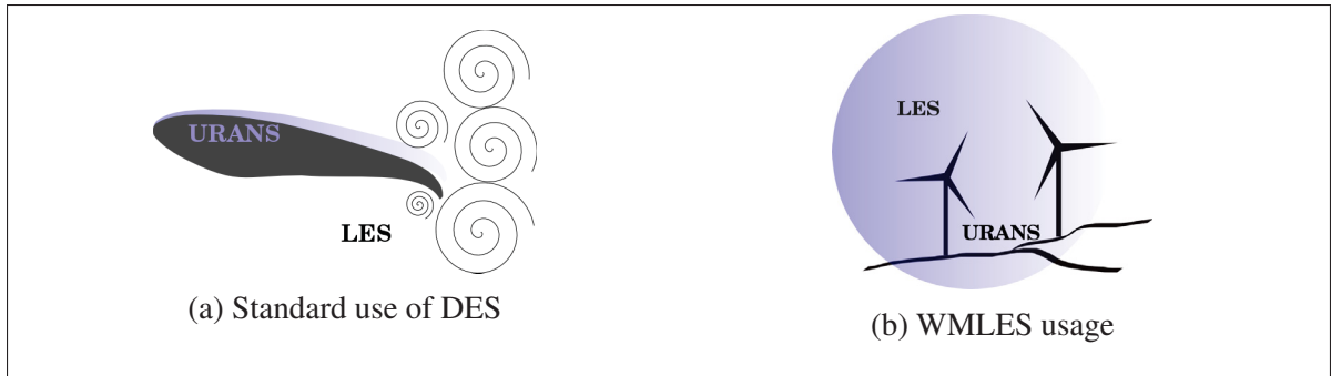
Figure 2.1 Sketch of DES applications. The extent of the boundary layer is represented by the colour blue. (a) The original DES was conceived to use URANS in the boundary layer, and LES everywhere else. (b) As a WMLES, the hybrid model employs URANS in the near-wall region, and LES far from the wall but within the boundary layer.
