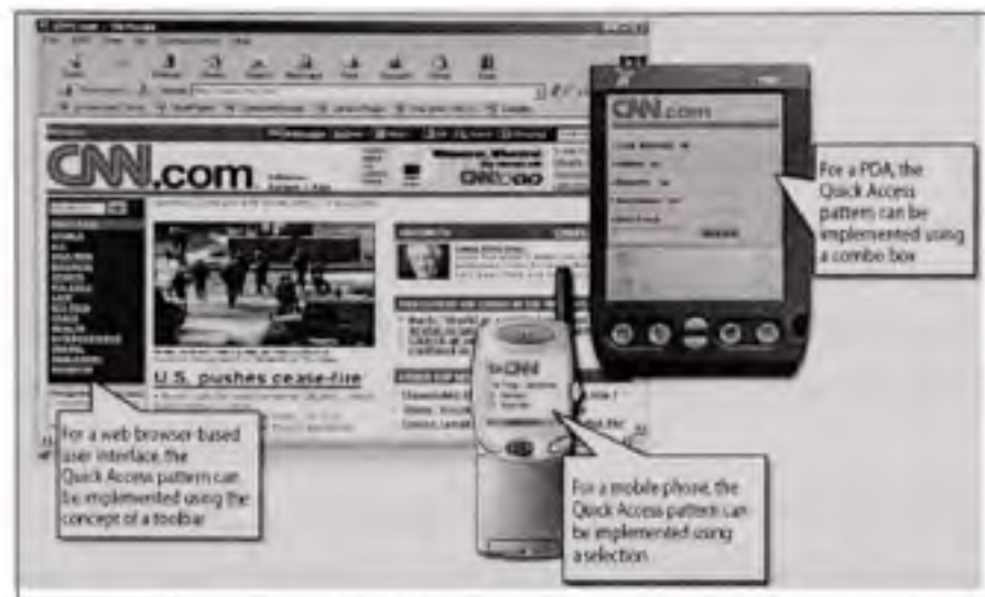
Figure 4.14 The Web Convenient Toolbar pattern implementations and Look and Feels for different platforms. (Extracted from the CNN Website)
