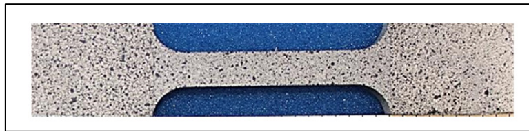
Figure 2-13 Speckle pattern on the measured surface
