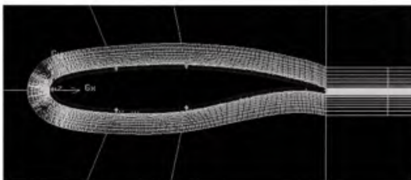
Figure 3.36 La couche limite permanente
