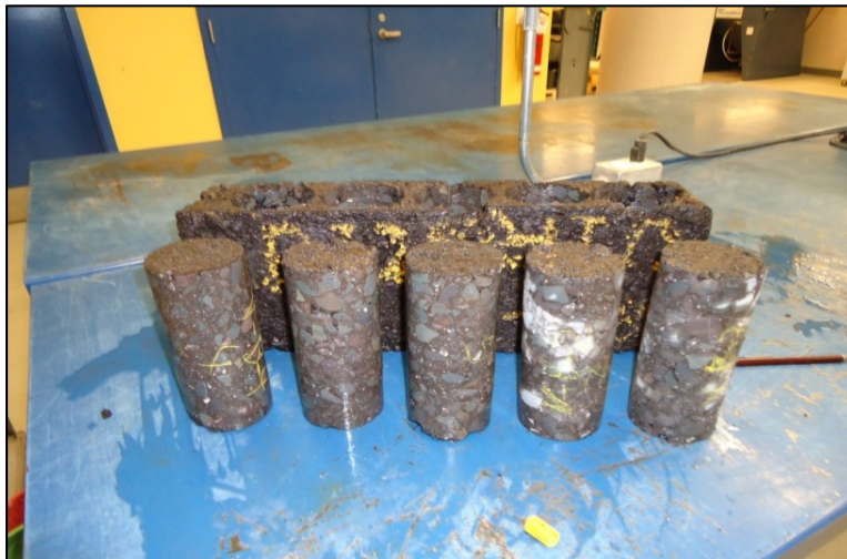
Figure 4.18 Five Cored cylindrical specimens of 75 mm diameter
