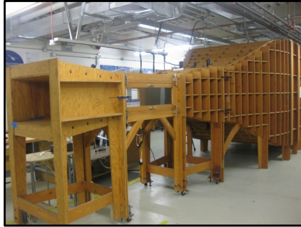
Figure 6.16 Price-Paidoussis wind tunnel
