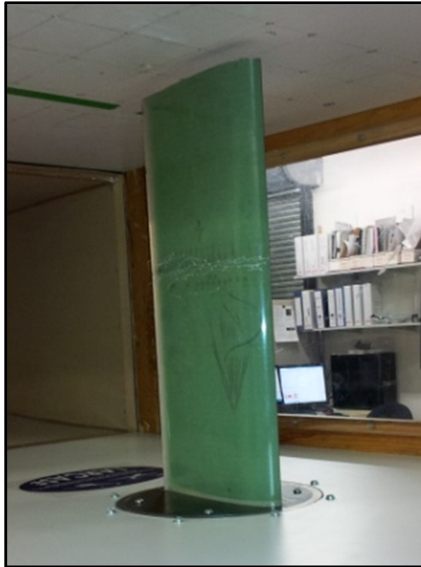
Figure 4.6 ATR-42 model installed in the test chamber of the wind tunnel
