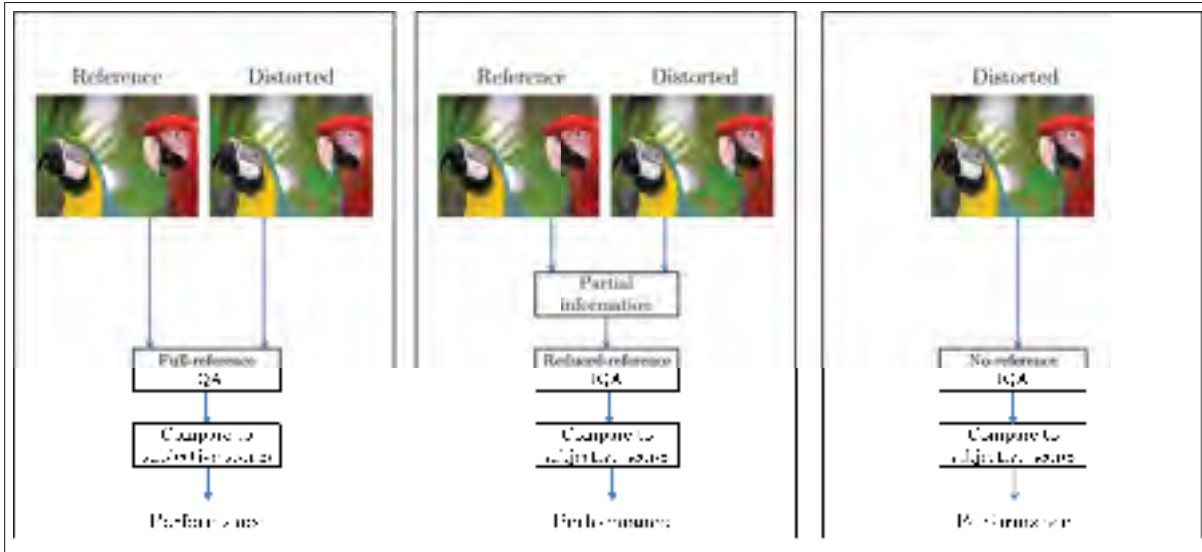
Figure 0.1 Category of image quality assessment models. From left to right, full-reference IQA model, reduced-reference IQA model, and no-reference IQA model.
