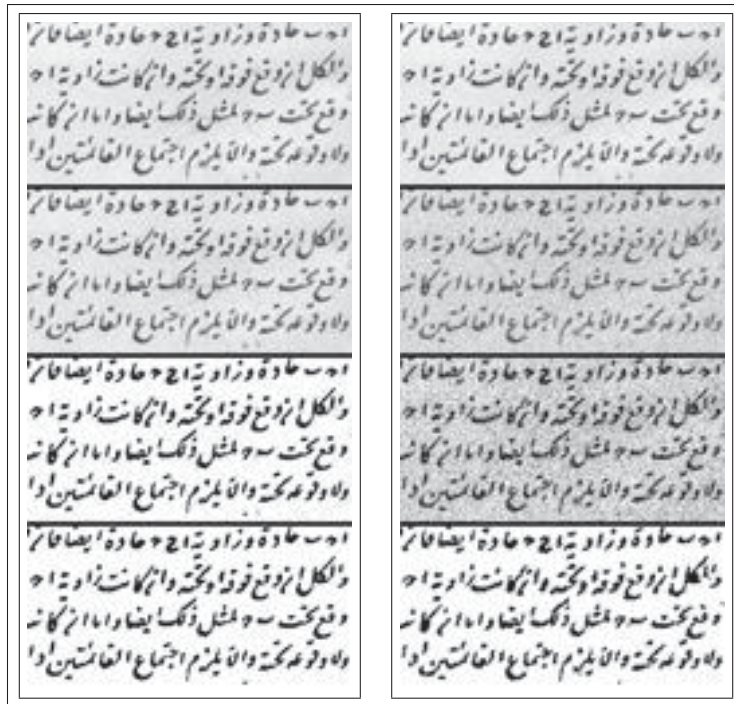
Figure 3.16 Pre-processing of image for keypoint extraction in the presence of noise, left) lower level of noise, right) higher level of noise
