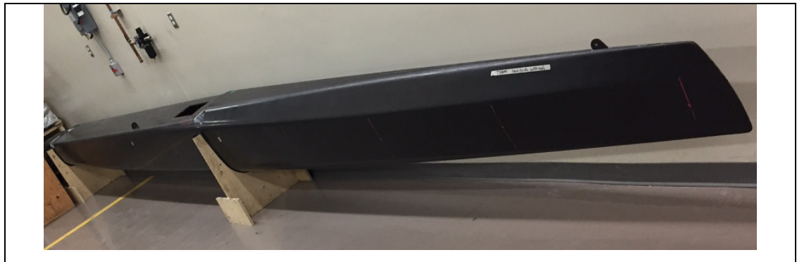
Figure 5.12 Coque tribord collée (avant finition)
