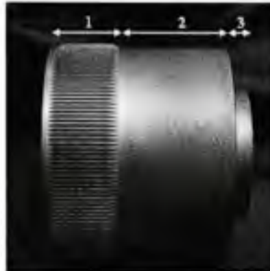
Figure 3. Side view of the flexspline showing the 3 studied portions
