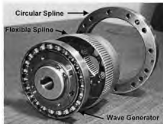
Figure 1: Typical components of a harmonic drive
