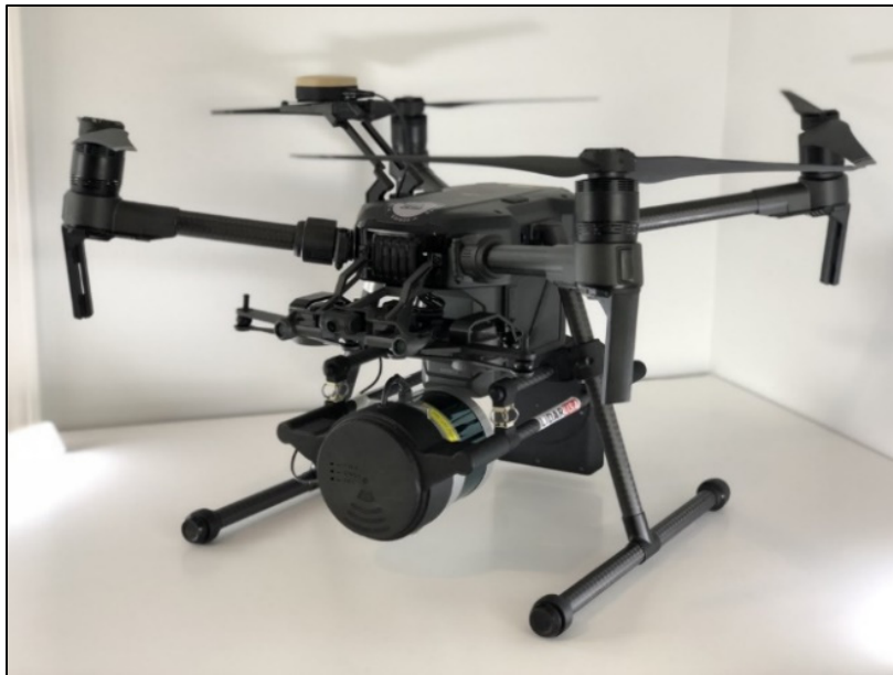
Figure 1.31 Can Drone M210 M8 Snoopy Lidar©
