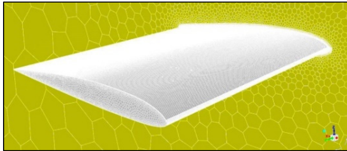
Figure 4.14 Mesh grid model of the UAS-S45 wing
