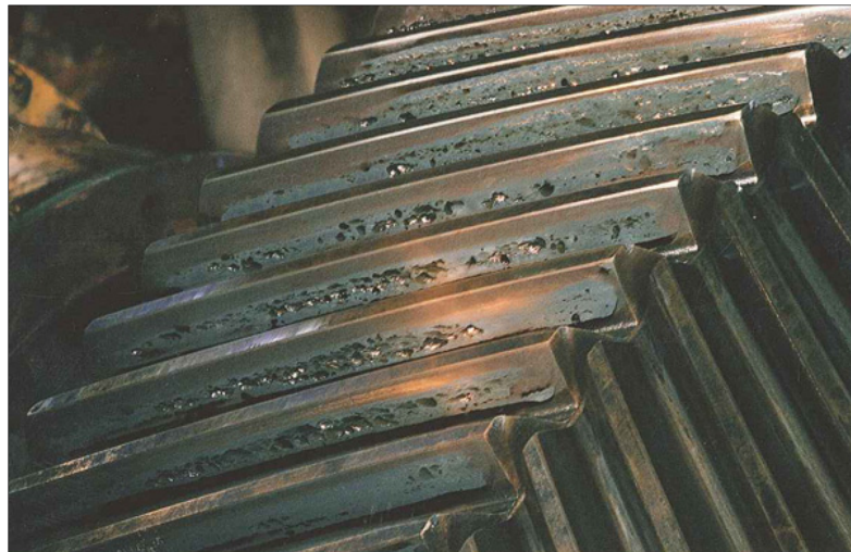
Figure 0.4 Pitting failure in a gear-Taken from (“Defects Treated (Gears) | Novexa,” n.d.)
