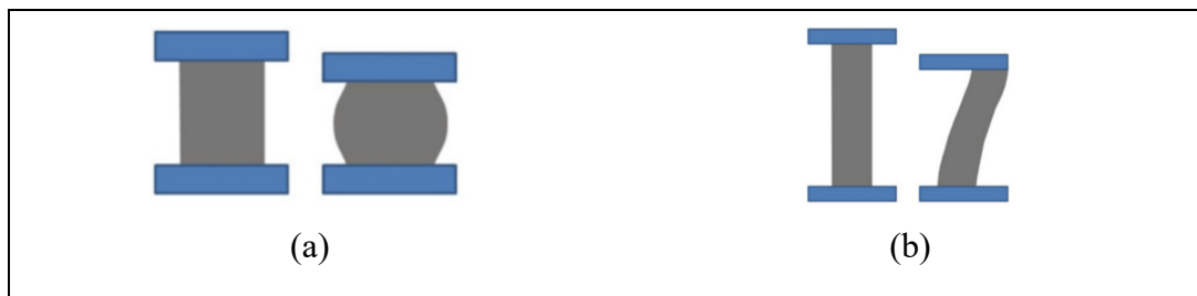
Figure 1.4 The deformation in the upsetting step of open-die forging: a) barreling and b) buckling Taken from Nee (2015, p. 181)
