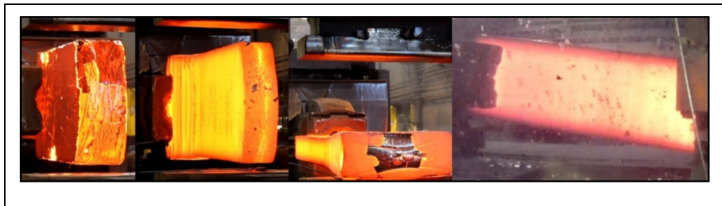
Figure 1.10 bringing the ingot to the desired geometry by finishing step
