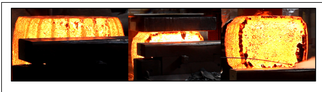
Figure 1.8 The FM phase in open die forging of large-sized ingots
