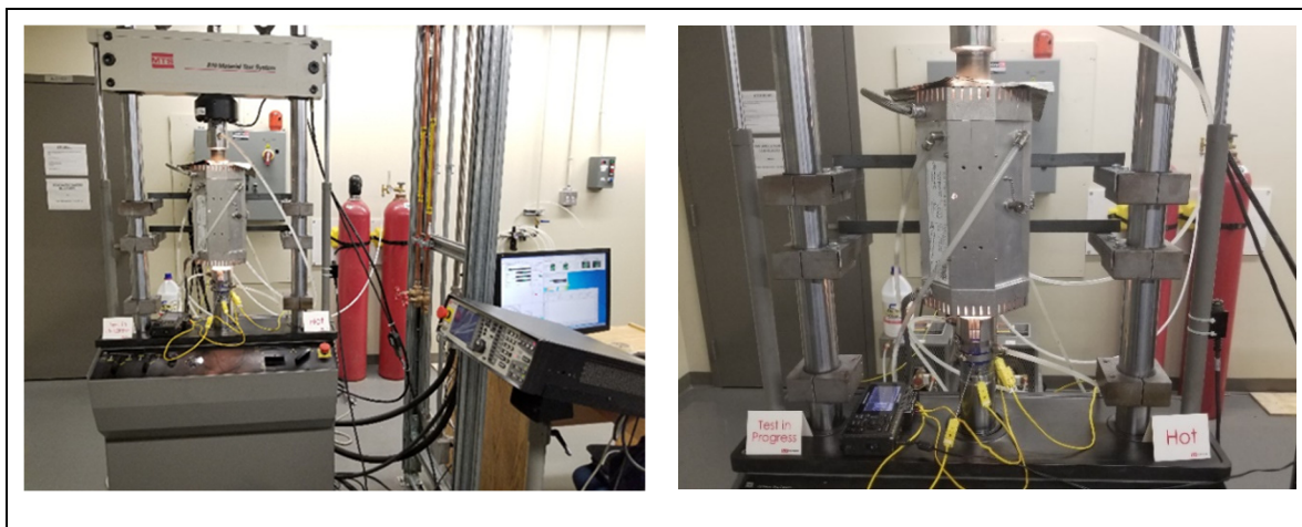
Figure 2.2 MTS machine with an installed radiative furnace
