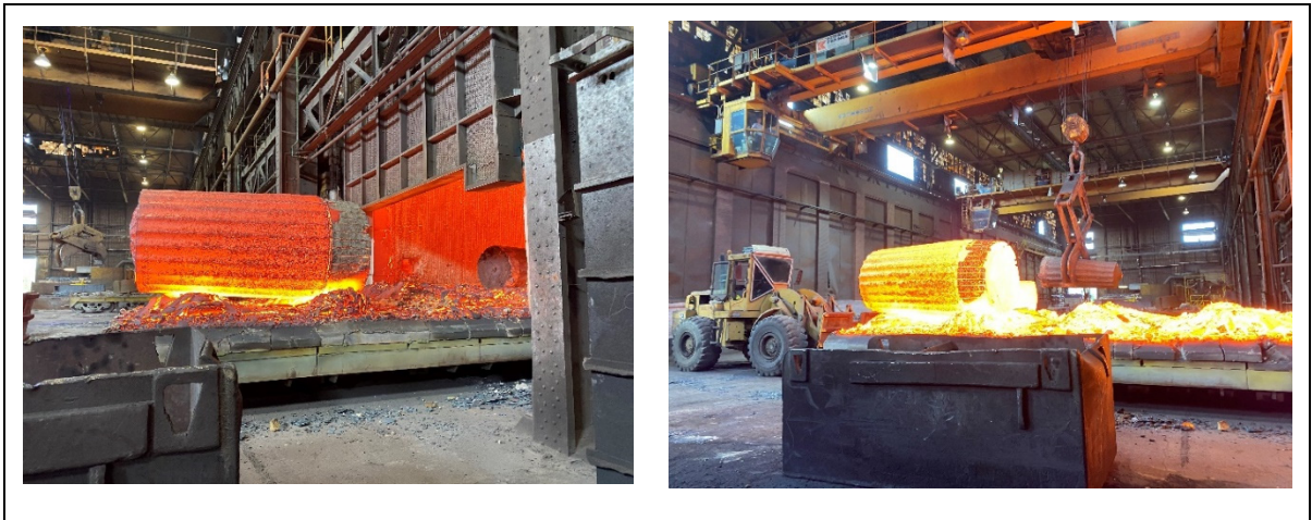
Figure 1.27 Heating large-sized ingots in gas-fired furnaces and transfer to forging by cranes
