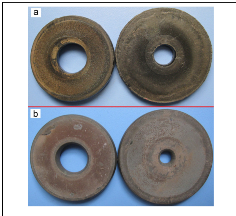
Figure 1.43 Deformed rings at 30% and 50% deformation for: a) glass lubricant, and b) dry friction Taken from Zhu et al. (2011, p. 2076)
