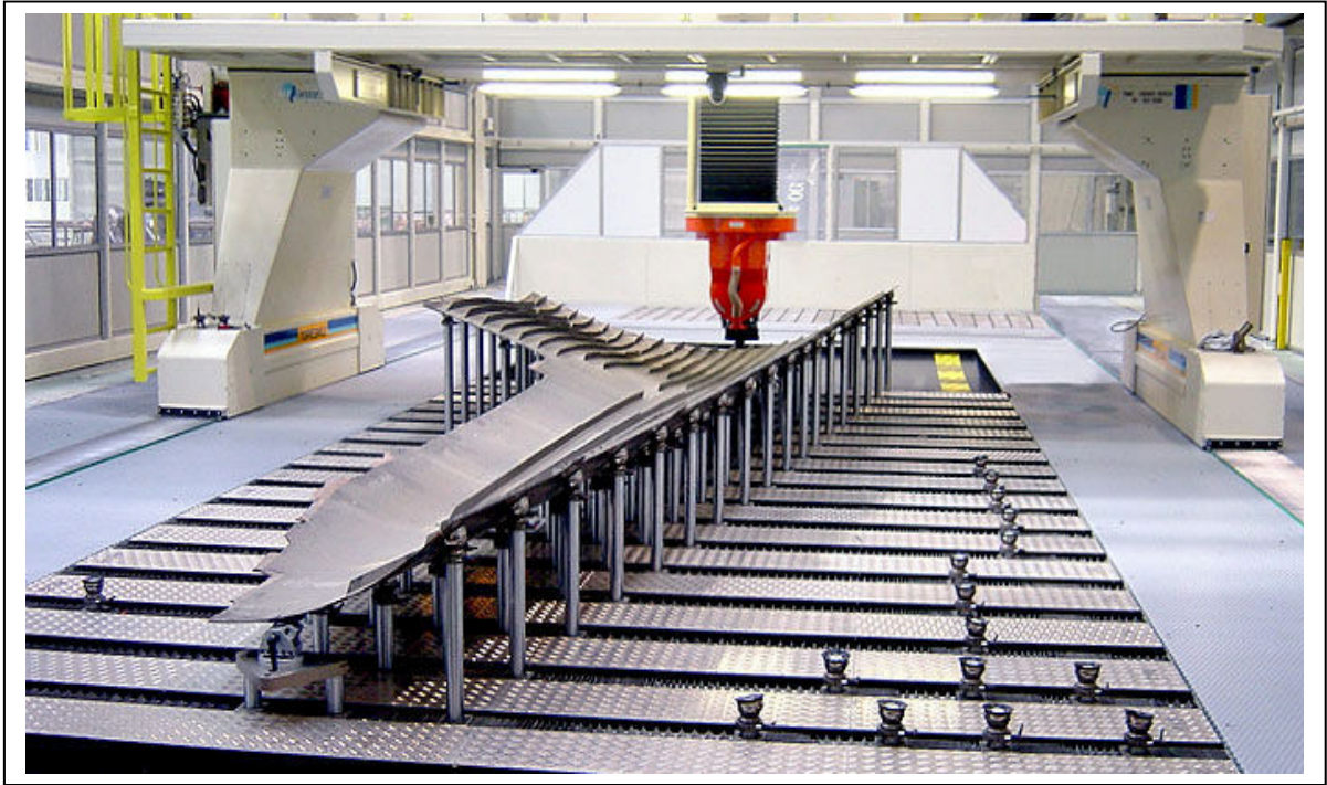
Figure 1-1 Flexible fixturing setup (MTorres, n.d.)
