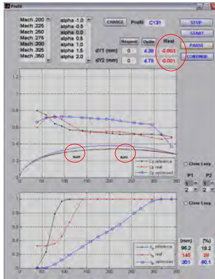
Figure 3.27 Results simulation for the airflow condition case C131 with the two actuators at the zero positions (0 mm).
