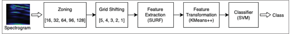
Figure 3.3 Overview of the proposed classification approach. Values in the first block indicate sizes of square zones (blocks) from 16×16 to 128×128. Stride values in the second block correspond to the zone sizes in the first block. For instance, a 96×96 block has stride 2, and so on.
