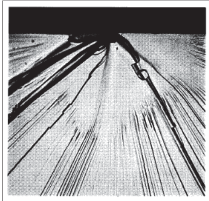
Figure 1.3 Fracture surface of cleaved single crystal germanium taken from Haneman et al. (1963, p. 2)
