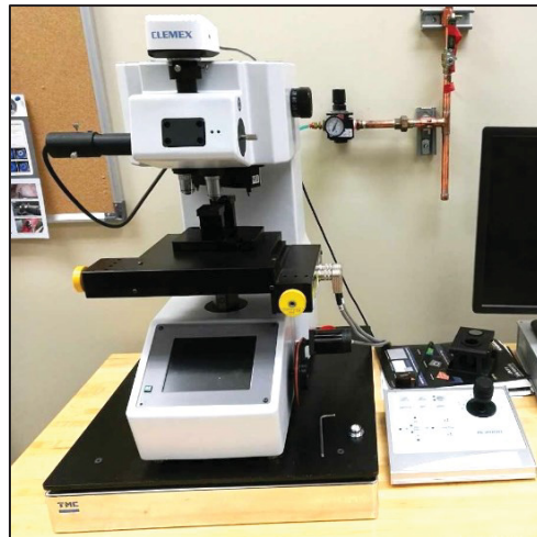
Figure 2.2 Photograph of the Clemex micro-indenter
