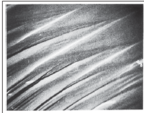
Figure 1.6 Detailed "V-shape" markings of cleaved Si taken from Kaufman & Forty (1986, p. 3170)
