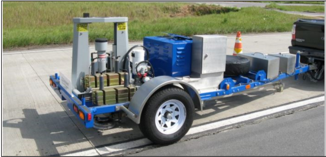
Figure 1.2 Typical FWD device Taken from FWD Transtec Group Inc. (2019)
