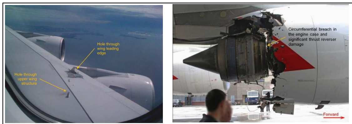
Figure 1.4 IPT Disc tri-hub uncontained failure on a Rolls-Royce Trent 972-84 Taken from Australian Transport Safety Bureau, (2013, p. 54, 258)
