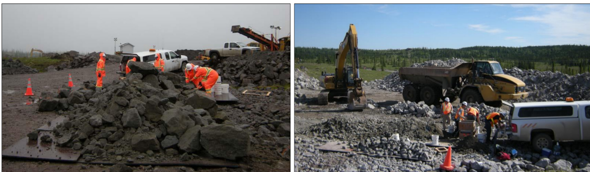
Figure 2.2 Carrying out a particle size analysis in the field. The left image shows how to measure the blocks, and the right image shows how to weigh them. Taken from Bouchard (2016)
