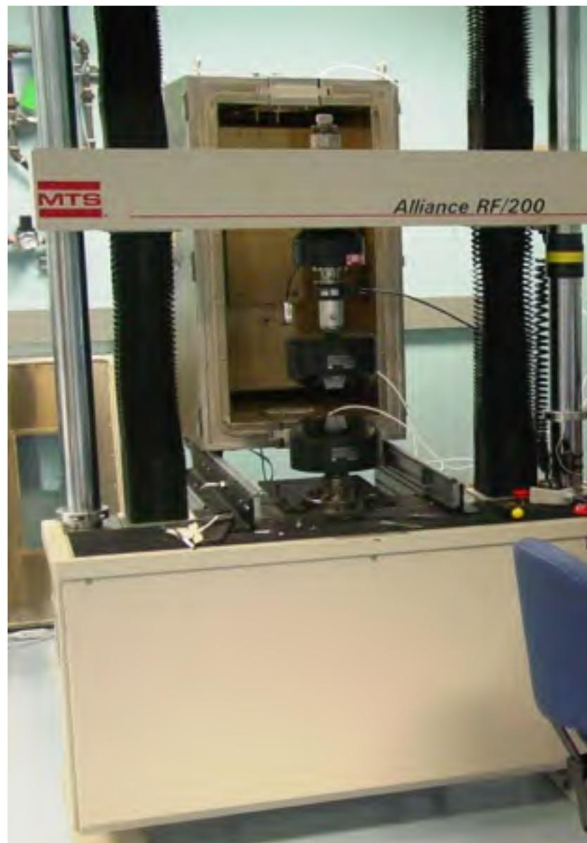
**Figure 2.8** Machine de traction Alliance RF/200
