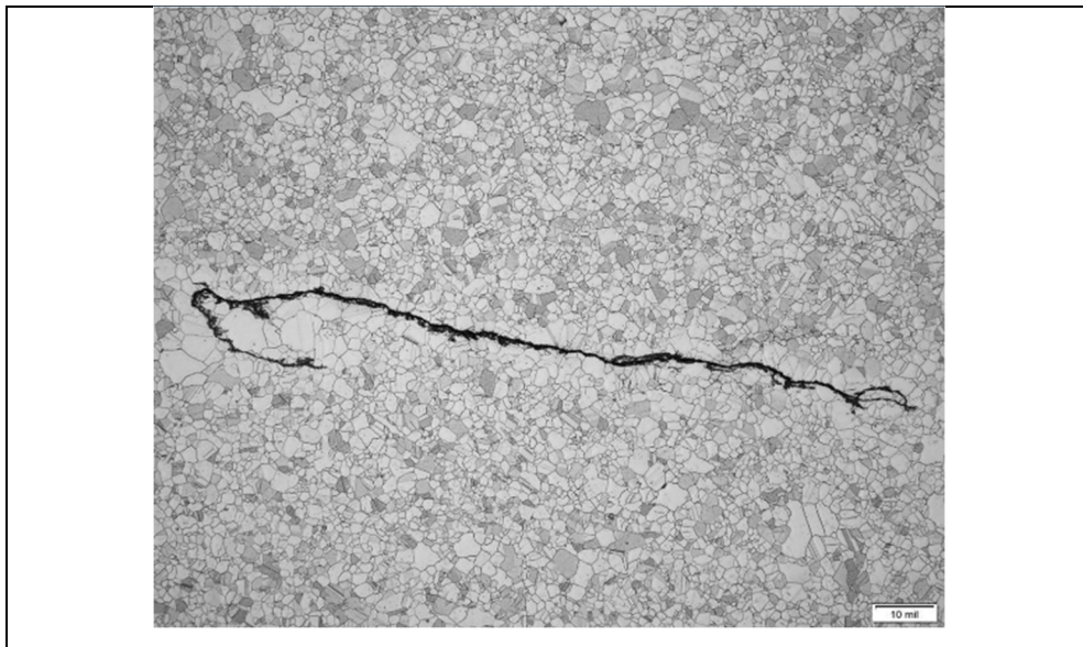
Figure 1-2 P&WC Waspalloy sample micrograph showing equiaxed microstructure and the presence of a crack
