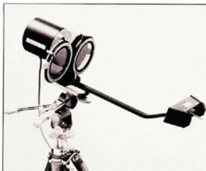
Figure 79 Montage du polariscope (Adapté de Photolastic Division measurement group, Inc., 1992)
