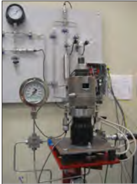
Figure 4.2 The stuffing box packing test bench.
