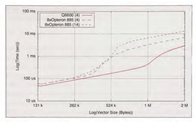
Figure 1.5: Execution time comparison between Intel's Q6600 and AMD's Opteron 885 processors. The concurrent process count is in parenthesis. The raw computing power of the Q6600 outperforms the Opteron 885 for four processes. The case of 14 concurrent processes is presented to demonstrate the proportionally small impact of their simultaneous execution.
