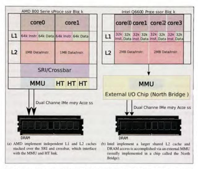
Figure 1.2: These schematizations of the AMD Opteron Dual Core processors (800 series) and the Intel Core 2 Duo processors illustrates how the two core variants access DRAM. In both cases, the MMU possesses dual channel connectivity to DRAM for link bandwidth aggregation.
