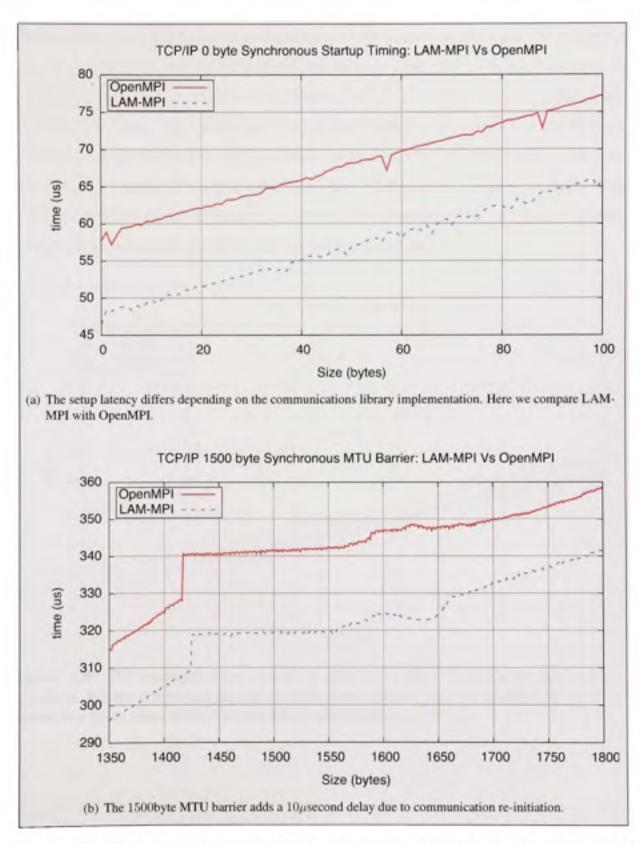
Figure 1.7: The round trip communication times using MPI libraries surrounding the start up times in (a) and the MTU in (b). Since these are round trip figures, all values have to be halved when considering asymmetric communication patterns.
