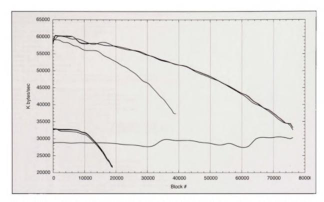
Figure III.2: The HDD's Zoned Constant Angular Velocity graph for 16 nodes of the *Thinkbig* cluster. These performance profiles illustrate well the heterogenety of the HDDs performance. The 40 and 80 G Byte HDDs start off with the same performance whereas the 20 G byte models are more than twice as slow.
