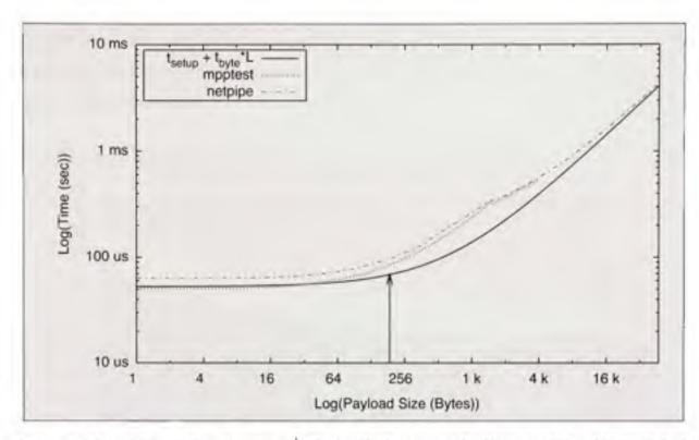
Figure 1.12: Comparing the general theoretical communications model with empirical values for a 100BaseT Ethernet network. Results from netpipe are slightly higher than mpptest, indicating there might be additional overhead to his test suite. The theoretical value bases its  $t_s$  on results from mpptest, thus biasing it to be closer to that tool's results. An arrow is inserted at 188bytes as a point of reference for a vector of 47 floats, a unit which comes in handy in our case study.
