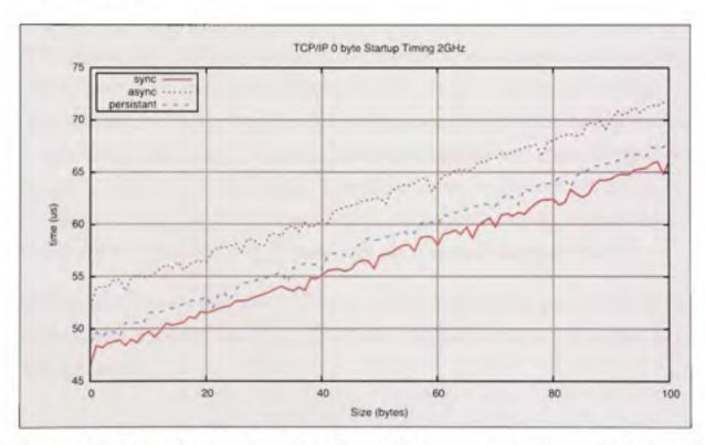
Figure 1.11: MPI call types and their impact on the communication times. Synchronous (sync) communications outperform both asynchronous (async) and persistant ones as the processor is dedicated to performing the communication task in that specific case.
