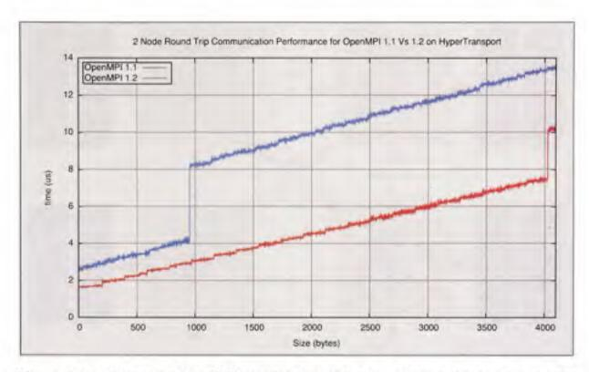
Figure 1.9: Comparing OpenMPI versions 1.1 and 1.2 on HyperTransport by varying the message size passed to the mpptest micro-benchmark. The 1.1 implementations had performance issues characterized by a sudden jump in communication times around packet sizes of 1000bytes.
