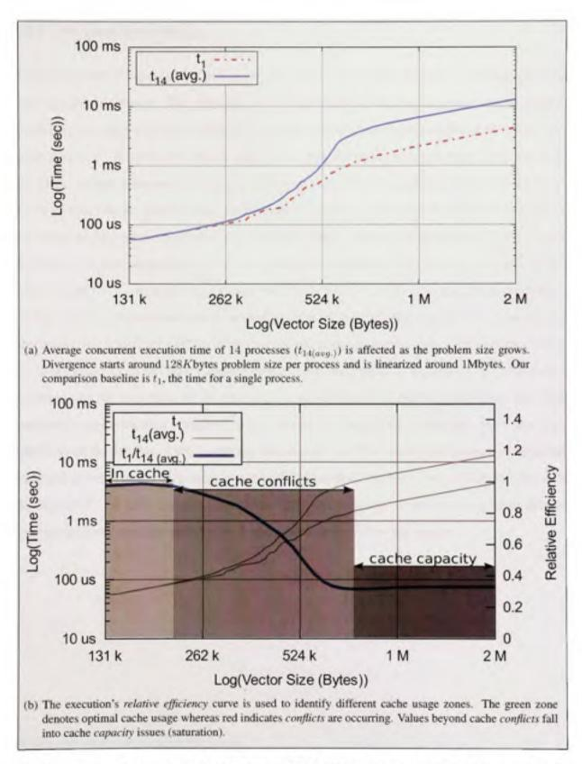
Figure 1.4: Cache memory behavior on AMD Opteron 800 series based processors using 14 cores of a SUN SunFire x4600. Execution time characteristics are illustrated in (a). Execution zones are identified in (b).
