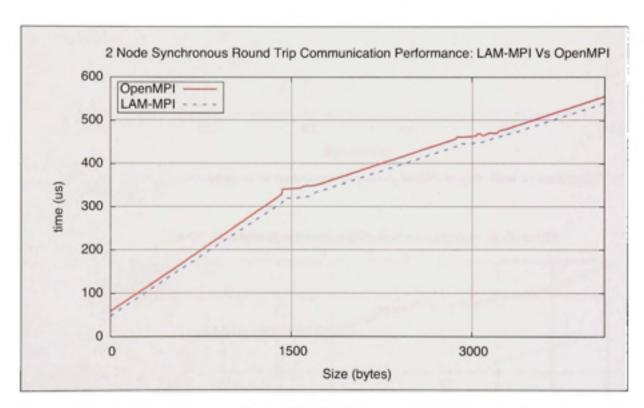
Figure 1.6: LAM-MPI outperforms OpenMPI for any TCP/IP communications. The non-linearity are noted around the MTU barriers of  $1500 \mathrm{bytes}$ .
