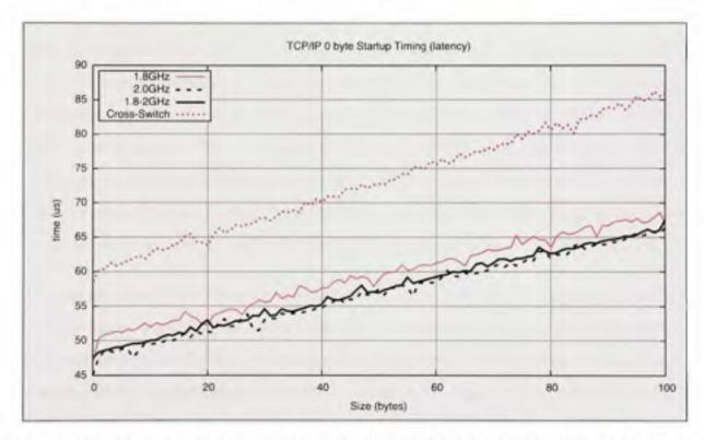
Figure 1.8: The communications latency is affected by the CPU frequency and network topology. Higher frequency clearly renders lower latency and the addition of a hop between two hosts (denoted as Cross-Switch) adds significant delays.
