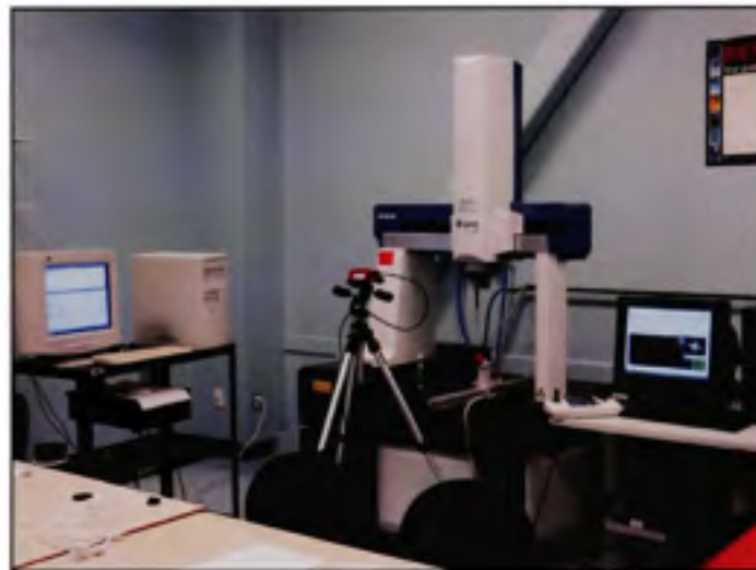
Figure 3.7 The experimental set-up for assessment of the error of positioning.
