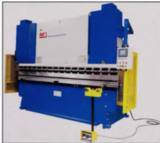
Figure 1.1 The hydraulic press-brake.
