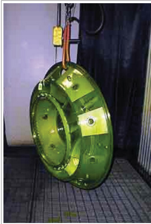
Figure 3.9 Draining station picture. Part of penetrant excess is drawn back to the penetrant application dip tank. This guarantees less penetrant waste, once part of the excess removed is reused.
