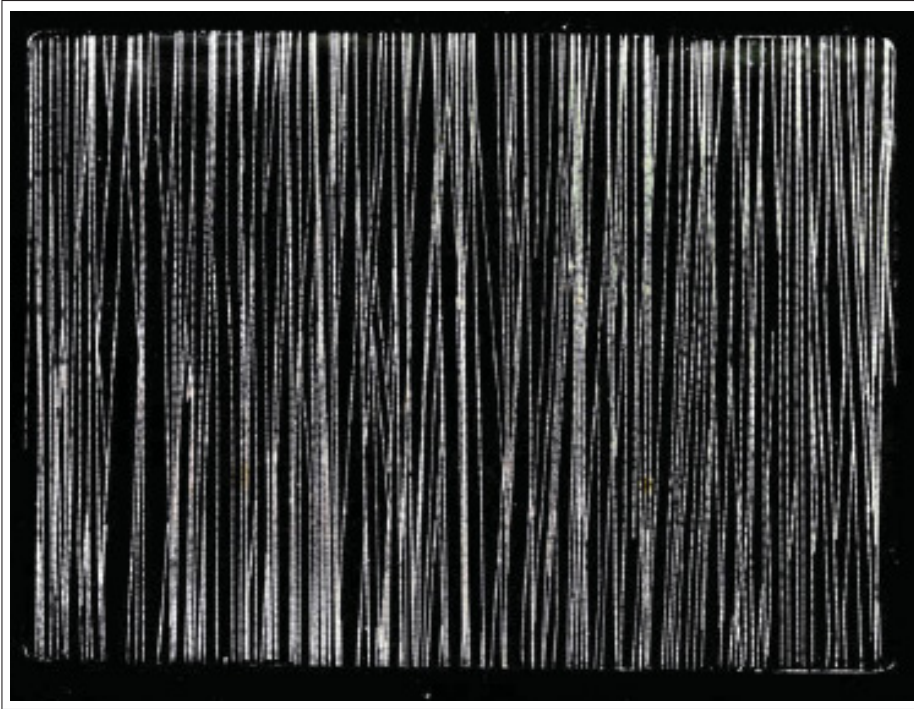
Figure 6.4 Radiography of Fine Test Panel containing open to surface cracks used to trace a POD curve.
