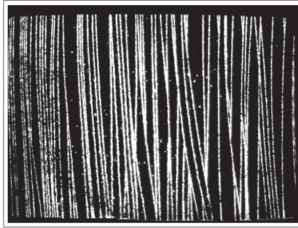
Figure 7.4 Image of the coarse sensitivity test panel that has been acquired through IDS . The angle \alpha and C have been set to 10^\circ and 30 centimeters respectively.
