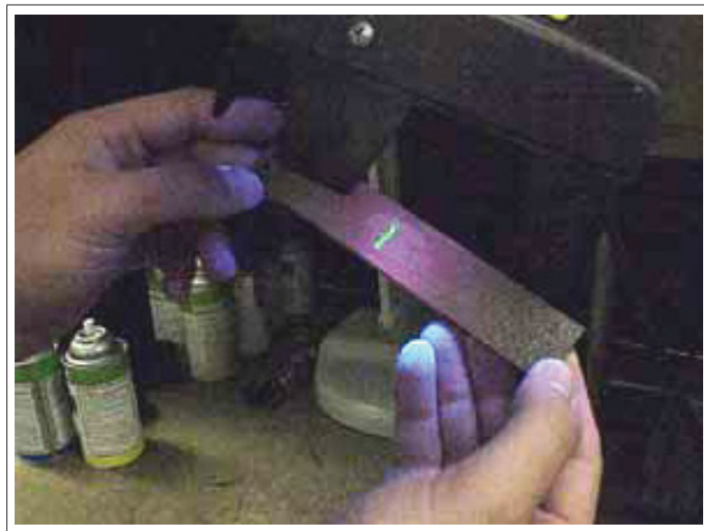
Figure 3.5 Inspection under UV light in a treated surface. Reproduced from NDT Resource Center (2010)
