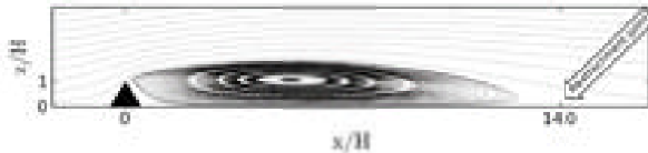
Figure 8: Time-averaged streamlines flow pattern around the triangular ridge.
