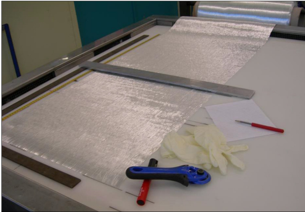
Figure 3.2 Cutting table and useful tools
