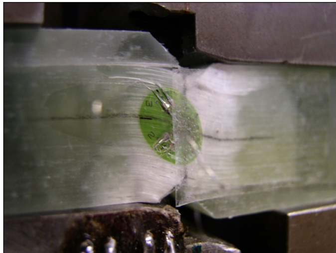
Figure 3.45 Example of a typical failure for an in-plane shear test of a UD V-notched specimen
