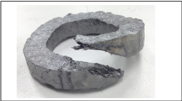
Figure 2.13 A flexible graphite plaited packing ring
