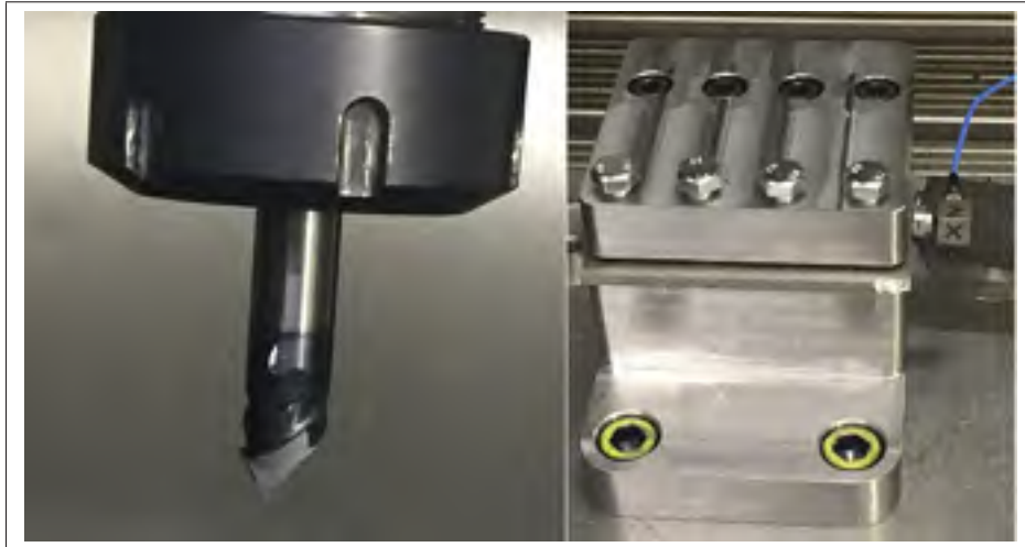
Figure 2.7 Tool breakage due to uneven surface of the workpiece in first path
