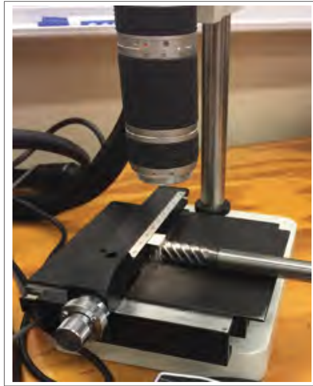
Figure 2.8 Keyence microscope used for tool wear measurement
