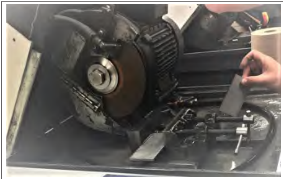
Figure 2.2 Work pieces are cut with wet saw
