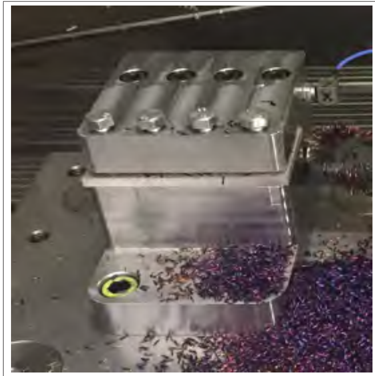
Figure 2.6 Jig designed for holding the work piece in place
