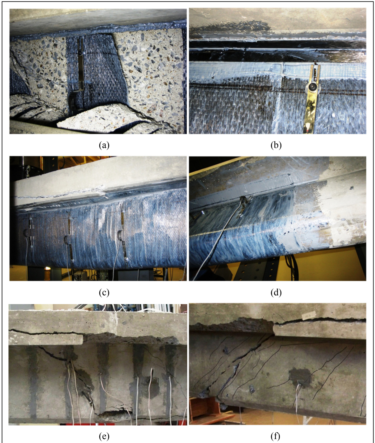
Figure 6.6 Strengthened specimens after failure: a) S3-EB-NA; b) S3-EB-SDMA; c) S3-EB-ERBA; d) S3-EB-EFLA; e) S3-NSM; and f) S3-EST.
