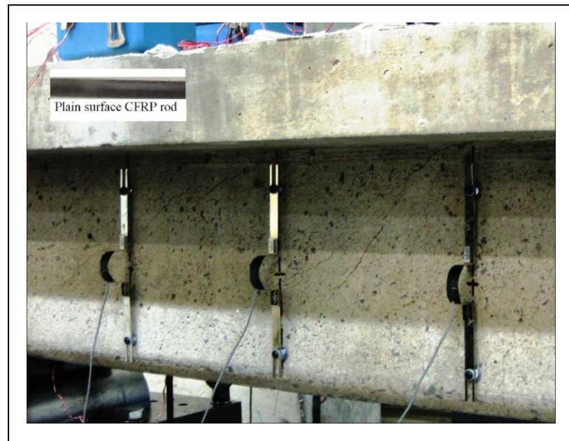
Figure 7.5 Parallel diagonal shear cracks, specimen S1-9d-260p.
