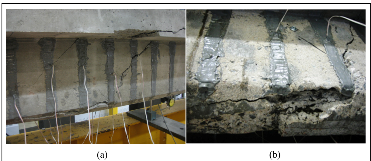
Figure 4.4 Common failure mode in beams strengthened with NSM method: a) Cracking pattern and b) detachment of concrete cover.
