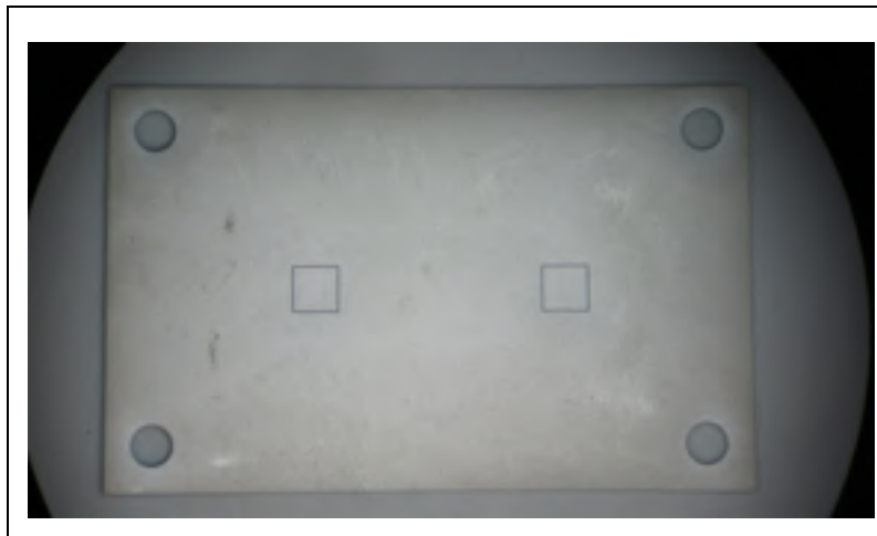
Figure 6.4 Top view: the slots of the two patches D in ground over substrate 9K7 Green Tape in LTCC
