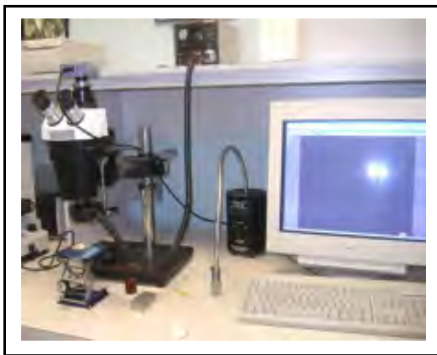
Figure 2.2 Optical microscope used for burr size measurement
