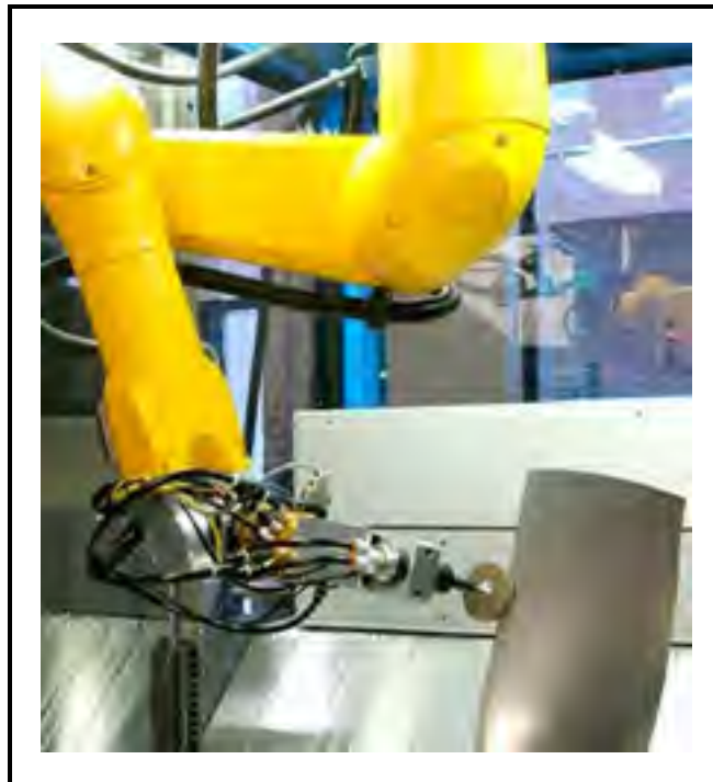
Figure 1.12 A robot arm combined with deburring brush (Means, 1986)
