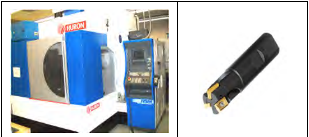
Figure 2.1 Experimental devices: (a) 3-Axis CNC machine (b) Cutting tool used
