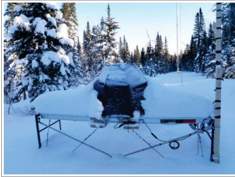
Figure 4.15 LiDAR on 2.5m platform deployed at AAV (Jeannotte et al. , 2011).
