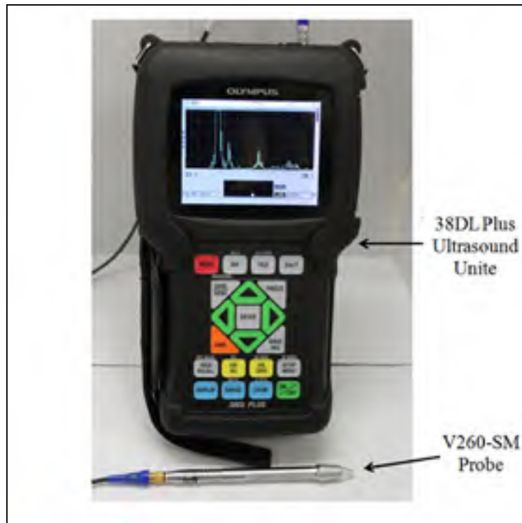
Figure 2.10: The ultrasonic thickness measurement device (38DL Plus)
