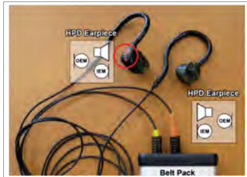
Figure 2.10 Sonomax ® earpiece from the individual dosimetric hearing protection with the emplacement of the microphone encircled in red adapted with the permission from Mazur and Voix (2013)
