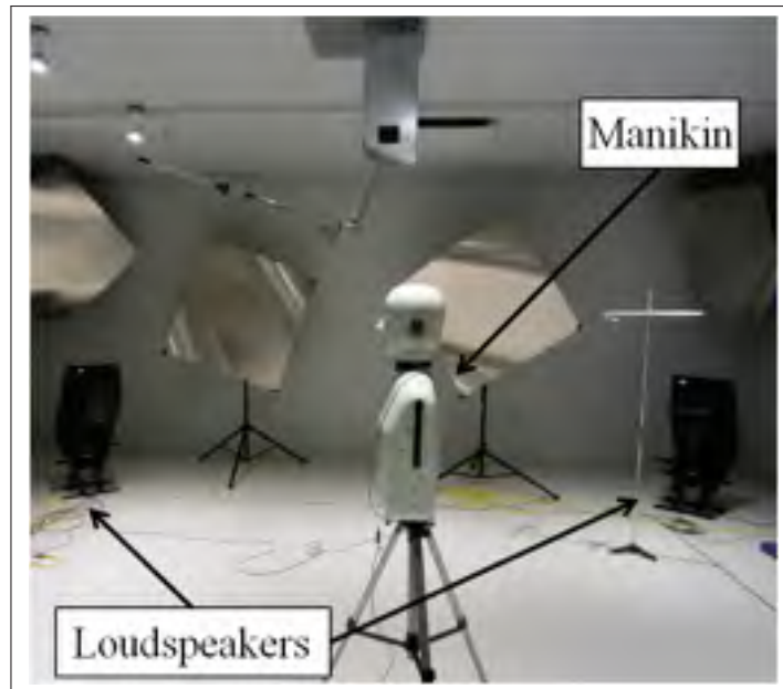
Figure 2.20 Measurement set-up in the reverberant chamber with the ATF located on the center of the reverberant chamber
