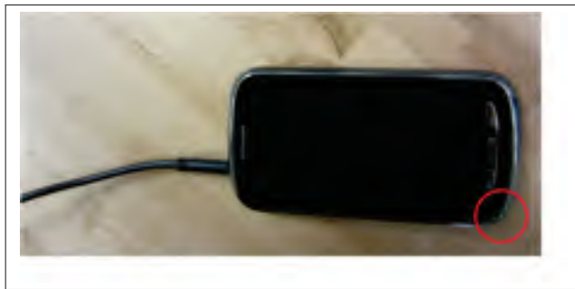
Figure 2.9 Unit of ZTE N762 mobile phone with the adapter cable plugged into the phone's audio input and the built-in microphone encircled in red
