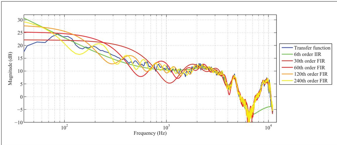
Figure 3.21 Frequency responses of IIR calculated from the truncated-transfer functions and frequency responses of FIR filters for orders from 30<sup>th</sup> to 240<sup>th</sup> order based on the initial built-in microphone transfer function
