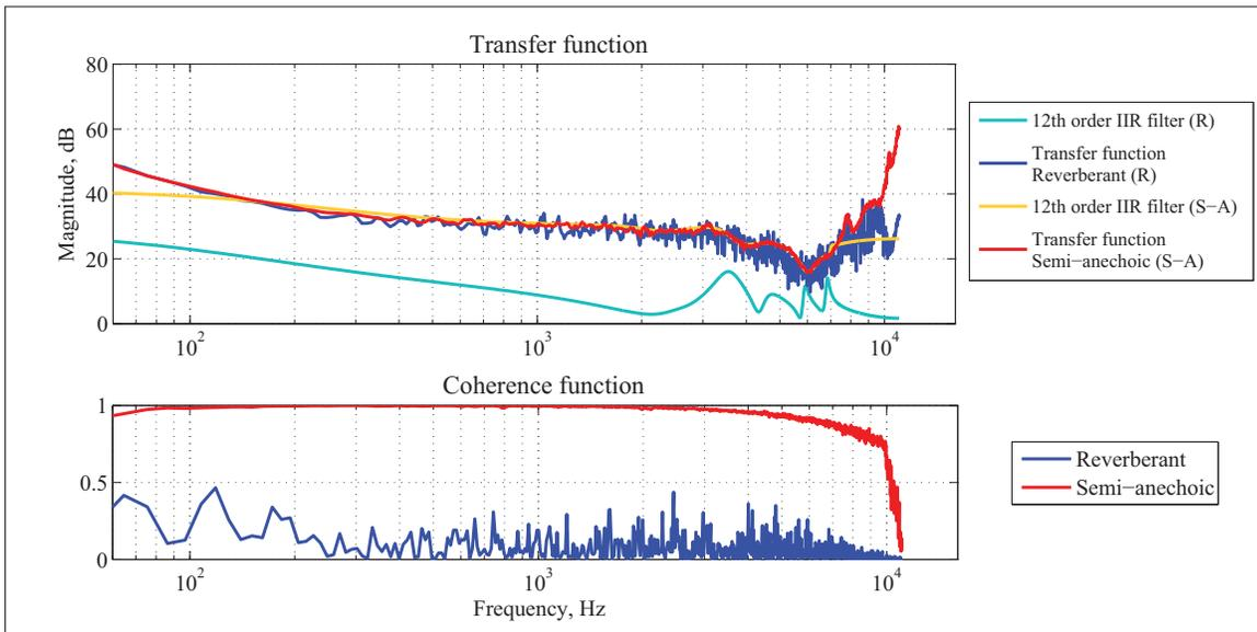
Figure 3.22 Earpiece transfer function and coherence values, frequency responses of 12<sup>th</sup> order IIR filters
