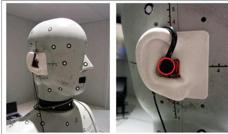
Figure 2.13 Sonomax<sup>®</sup> earpiece on the ATF's built-in ear simulator with the location of microphone encircled in red
