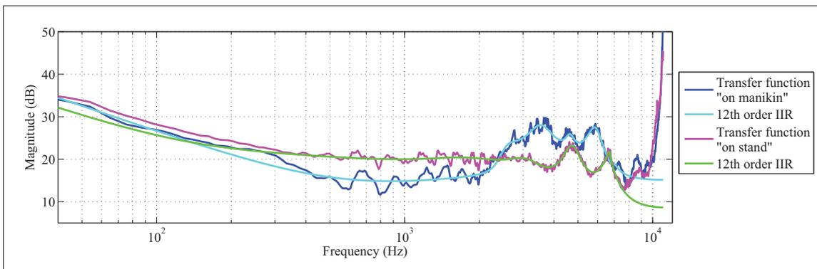
Figure 3.18 Headset transfer functions based on the measurement for different microphone placements and frequency responses of the 12<sup>th</sup> order IIR filters, calculated from the truncated-transfer functions (from 43 Hz to 7250 Hz)
