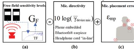
Fig.1. Calculation of the *calibration adjustment* with the field calibration values; assessing free-field mic. sensitivity relative to calibrated device (a), then accounting for mic. directivity (b) and mic. placement position (c).
