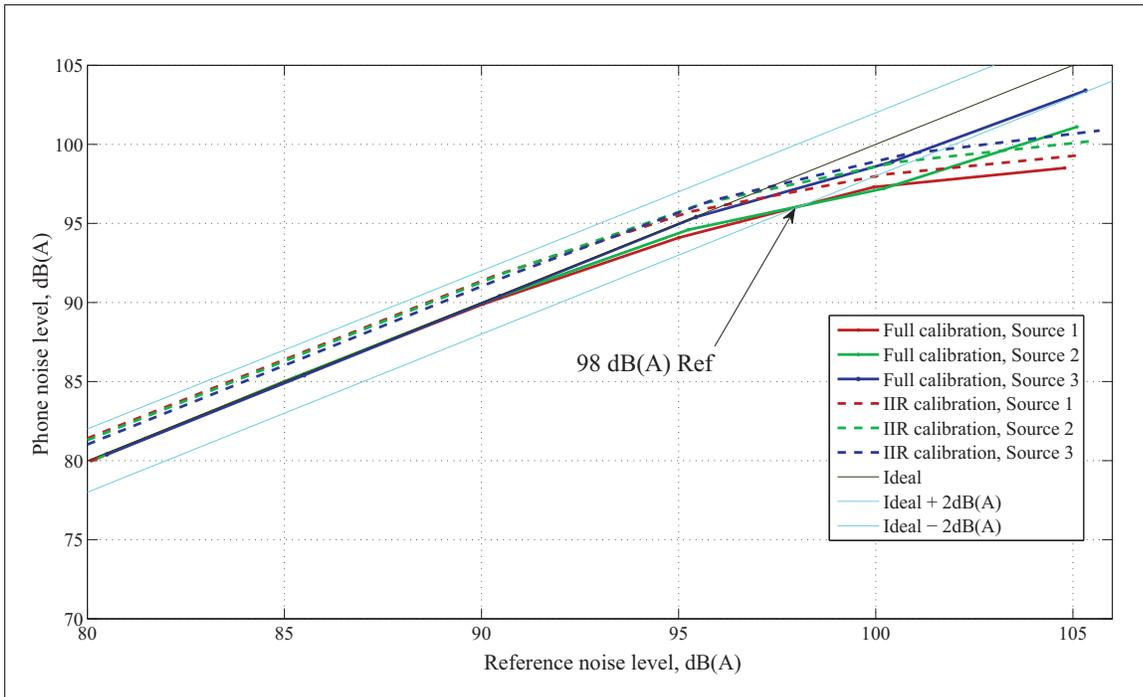
Figure 3.33 Built-in microphone noise level measurements in the **reverberant** chamber with only a frequency-dependent calibration (FIR calibration) and with frequency and level-dependent calibration (Full Calibration)
