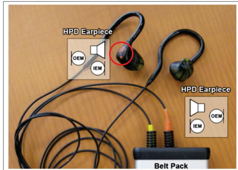
Figure 2.10 Sonomax<sup>®</sup> earpiece from the individual dosimetric hearing protection with the emplacement of the microphone encircled in red adapted with the permission from Mazur and Voix (2013)
