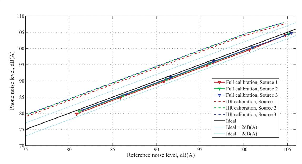
Figure 3.29 Headset noise level measurements carried out in the **semi-anechoic** chamber, with only a frequency-dependent calibration (IIR calibration) and with frequency and level-dependent calibration (Full Calibration)
