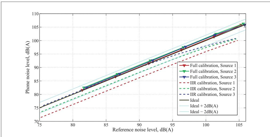
Figure 3.36 Earpiece overall A-weighted errors measured in the **semi-anechoic chamber** with only a frequency-dependent calibration (*FIR calibration*) and with frequency and level-dependent calibration (*Full Calibration*)
