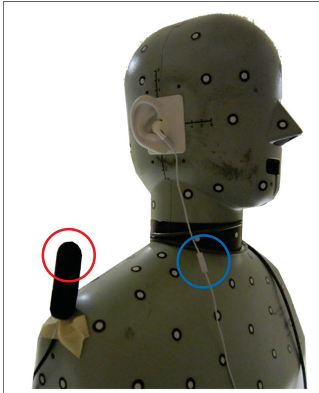
Figure 2.14 Placement of the Apple iPhone<sup>®</sup> headset microphone (encircled in blue), and the standardized noise dosimeter (encircled in red) on the ATF
