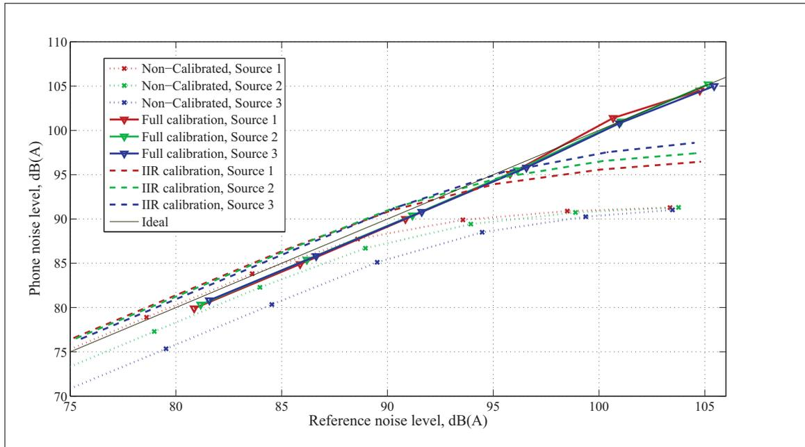
Figure 3.32 Built-in microphone noise level measurements in the **semi-anechoic** chamber without calibration, with only a frequency-dependent calibration (IIR calibration) and with frequency and level-dependent calibration (Full Calibration)
