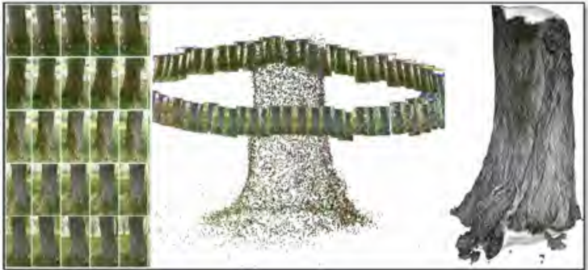
Figure 2.4: Three-dimensional reconstructions by image base modeling and Structure from Motion (SfM). Left: overlapped sequential images, Middle: Camera position and Camera path & direction in image recoding, Right: Textured mesh of object. (Horning, 2012)
