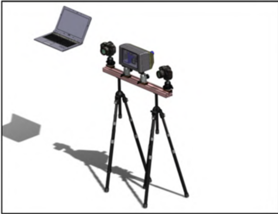
Figure A. 6: Validation prototype Concept design
