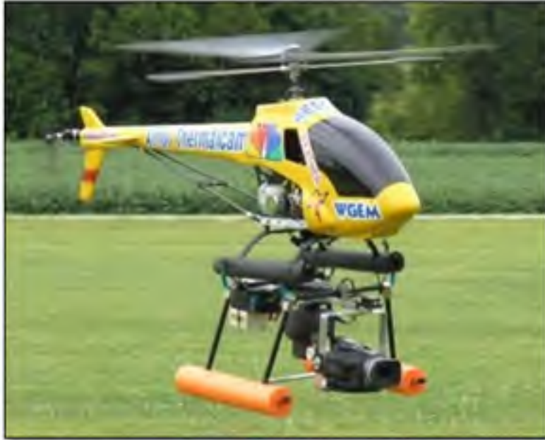
Figure 3.27: Remote controlled Helicopter for WT image acquisition (Source: http://www.airfoilsycam.com )
