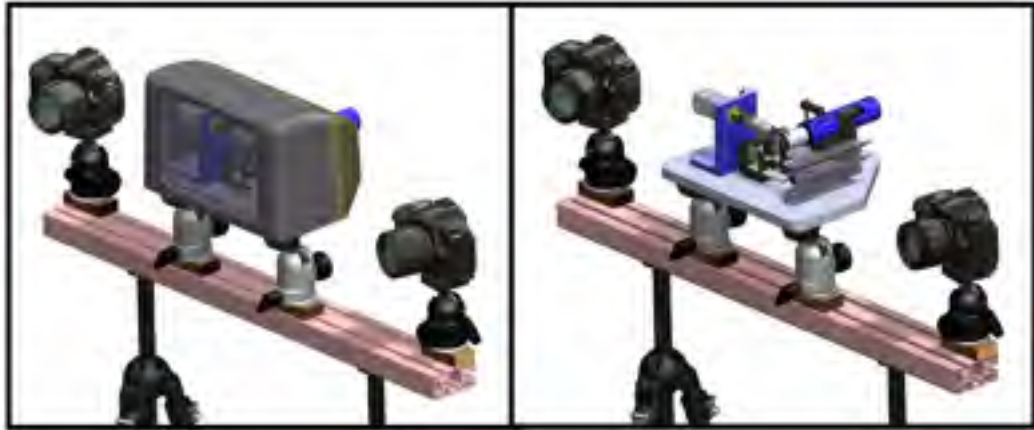
Figure 2.7: Customize laser scanner equipped by laser beam at wavelength 405-460 nm
