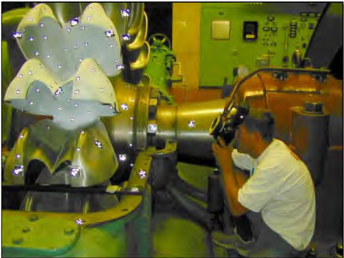
Figure A. 15: Ring flash on DSLR camera helps to illuminate from viewing direction of camera, source: www.capture3d.com .
