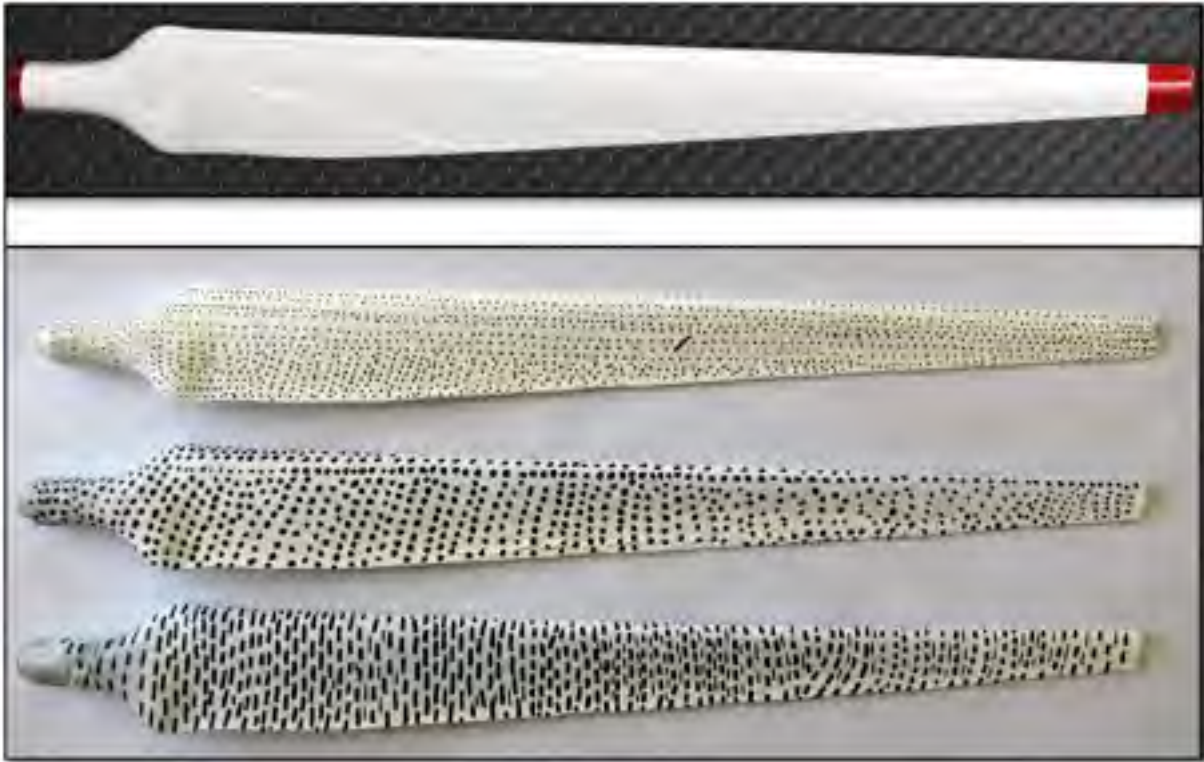
Figure 3.20: Up: Render view of Master CAD data, Down: Prototype blades with different surface patterns and targeting layout, From top Pattern 1 to 3
