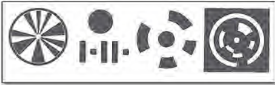
Figure A. 14: Selection of coded targets (bit series)
