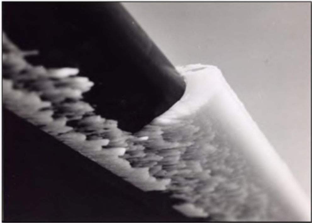
Figure 1.3: Aircraft Propellers with accumulation of precipitation ice on leading edge, image taken between 1969-73, in Sea-king, Wessex. Ontario Canada. (source: www.eacott.com.au/gallery/d/3366-1/icing+4 )
