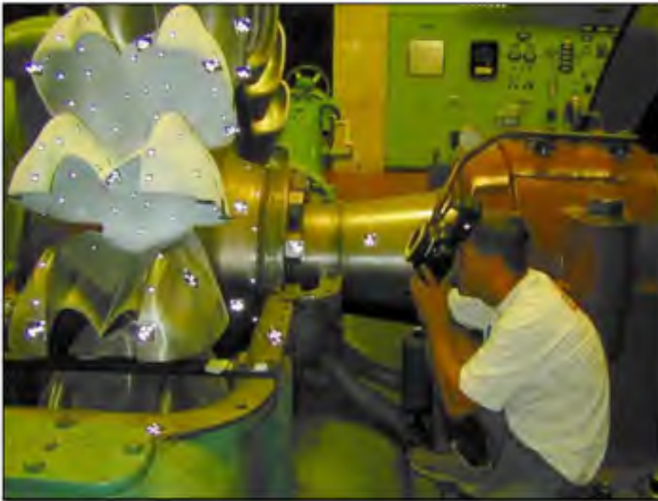
Figure 3.5: Ring flash on DSLR camera helps to illuminate from viewing direction of camera, source: www.capture3d.com
