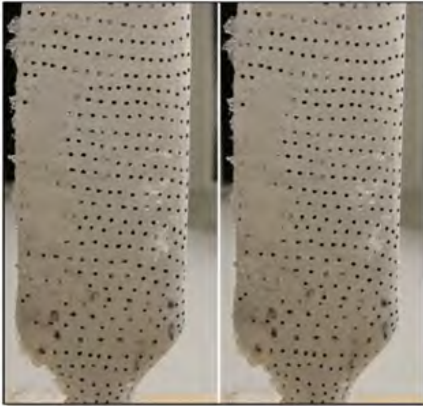
Figure 3.15: Left: Original Photo, Right: Rectified Photo from Same photograph, distortion corrected
