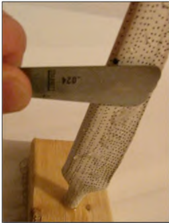
Figure 4.16: Manual measurement of iced region. Filler gauge shows \approx 2.9\text{ mm} in area
