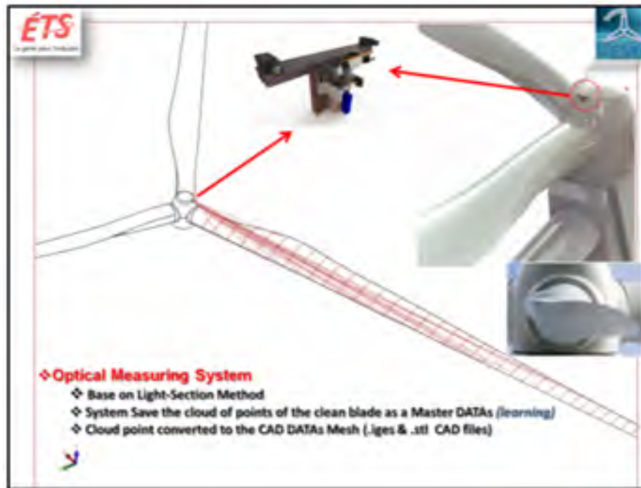
Figure A. 4: Installation position of system on the Wind Turbine Hub
