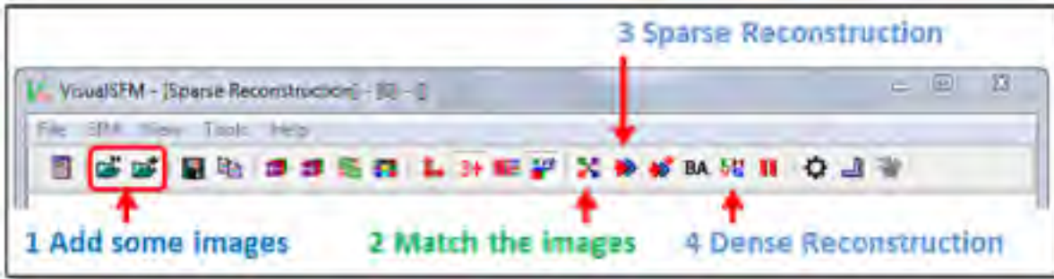
Figure 3.16: 3D Reconstruction - Using the VisualSfM GUI
