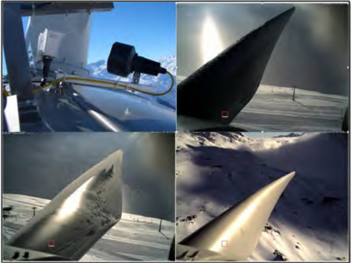
Figure 1.7 : (Top left) Installed camera on the Nacelle, the lamp on the right is for heating purpose. (Top right) rime ice observed on the blade. (Bottom left) rime ice after 45min heating system on, (bottom right) de-iced blade, some little trace of glazed ice remained on the leading edge. Source : (Cattin, 2015)
