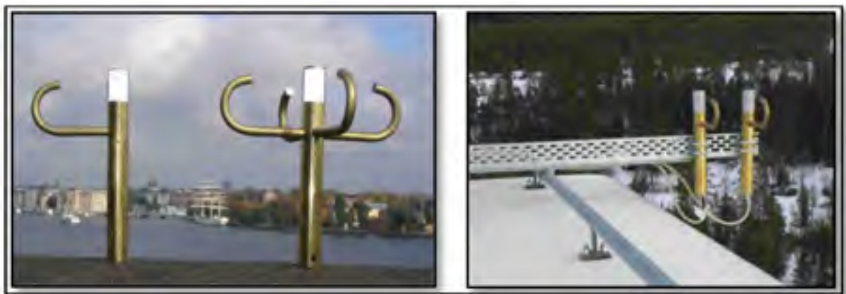
Figure 1.5: (Left) T23 & T26 Icing Rate Sensor, (Right) T41 shown on the nacelle at the wind power plant in Härnösand, northern Sweden. Source: HoloOptic.net
